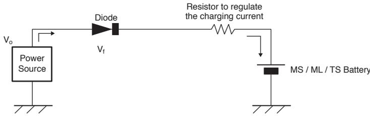
The charging voltage “Vo” must Not be higher than 3.3V (MS series) / 3.1V (ML414H) / 3.0V (TS series).
