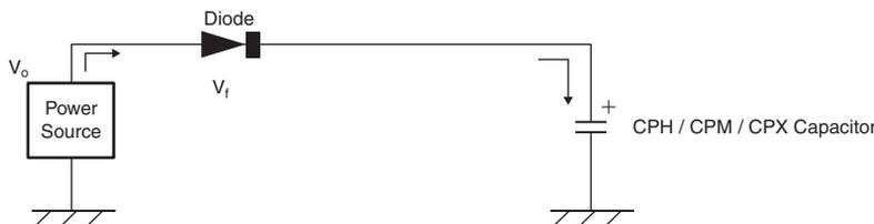
You do not need to insert a resistor to regulate charging current.
