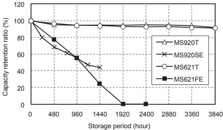
MS-T series' capacity retention ratio after High temperature storage were greatly improved.
