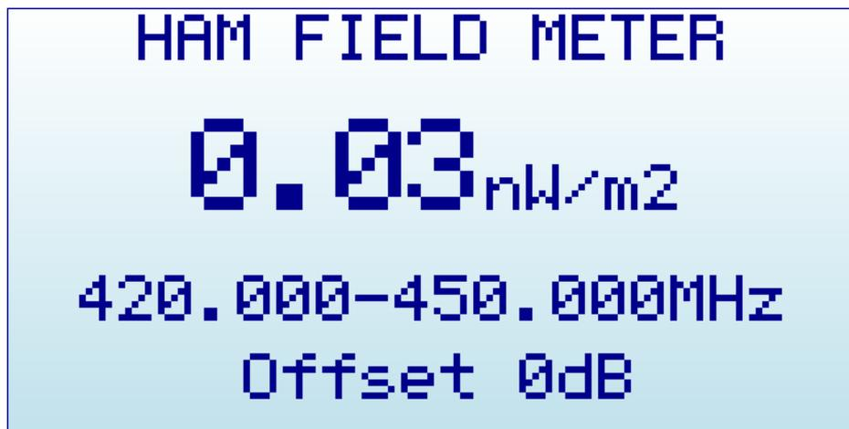
Measurement values are automatically scaled and adjusted to pico/nano/micro/milli for convenient screen reading.
