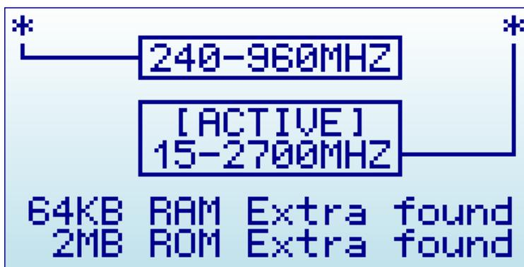
**Important:** Only one of the two SMA connectors is enabled at any given time. You select the active one using the Module option in the Frequency Menu, see page 16.
