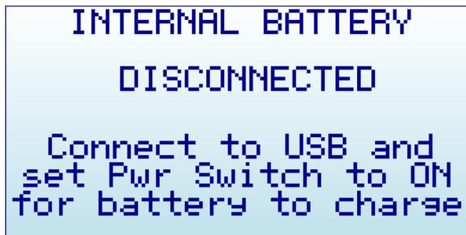
As soon as the power switch is set to the correct position, the screen will display correct charging status.
