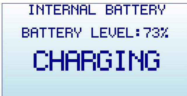
At this point you can close this screen pressing ENTER or RETURN. If you keep it active for more than 15 seconds, it automatically sets the device in SLEEP MODE - all internal circuits and LCD backlight go off, except for charging and minimal CPU monitoring - This is the recommended procedure to charge the device
