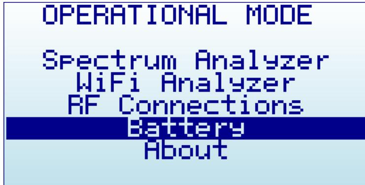
Use [Up] and [Down] arrow keys to select the desired mode and click on [Enter] to activate it immediately.
