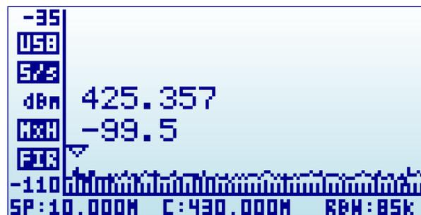
In this screen above, the frequency reading at the bottom changed from Start/Center/Stop frequency to Span/Center/RBW. When this mode is enabled, a key press on [Left] or [Right] button will increase or decrease to double and half frequency span respectively.
