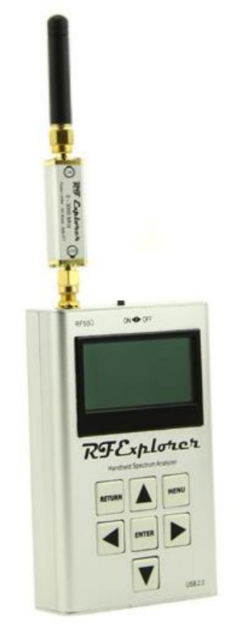
The RF Explorer Power Limiter will allow any RF Explorer model to be protected with external signals up to +30dBm (1 Watt), so you get the same level of protection as in the WSUB3G. Furthermore, the power limiter includes additional functionality inside that will otherwise require external devices increasing cost and size:
