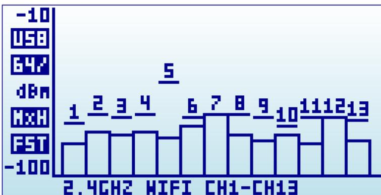
The same setup described before, but inspecting the activity for a longer time, shows the channel 5 is the one with higher level detected, so we confirm is not a good choice.
