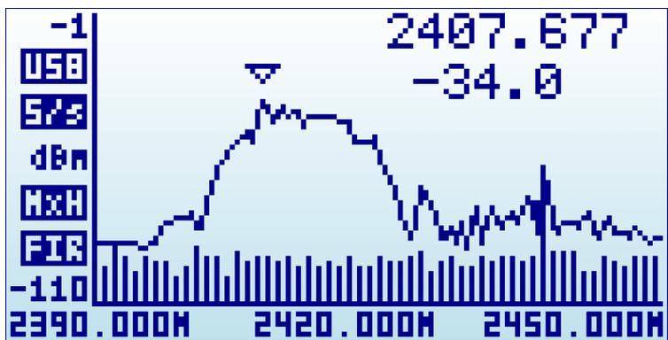
The X axis represents frequency in MHz and Y axis display actual received power in dBm or dBuV (selectable). In this example above, the frequency span goes from 2390 MHz to 2450 MHz (that is a 60MHz range), and the visual amplitude goes from -1 dBm to -110 dBm.
