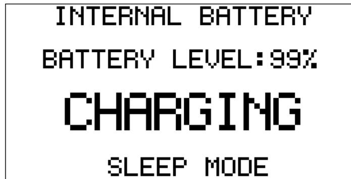
In this mode you can stop charging whenever the device reaches 99% or 100%, which may take up to 2 or 3 hours under normal condition and depending on initial battery charge level. When the charging algorithm detects the battery fully charged and a minimum of 2hs connected, it will suggest disconnecting the USB cable.
