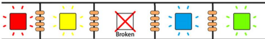
Digital RGB LED Flexi-Strip is an intelligent light source consists of WS2813B RGB LED with Integrated Driver Chip. The control circuit and RGB chip are integrated in a package of 5050 components.
