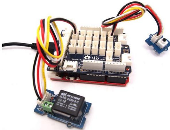
Below is a demo that shows you how to control a Grove - Relay with a Grove - Button. When the button gets pressed, the relay will close.
