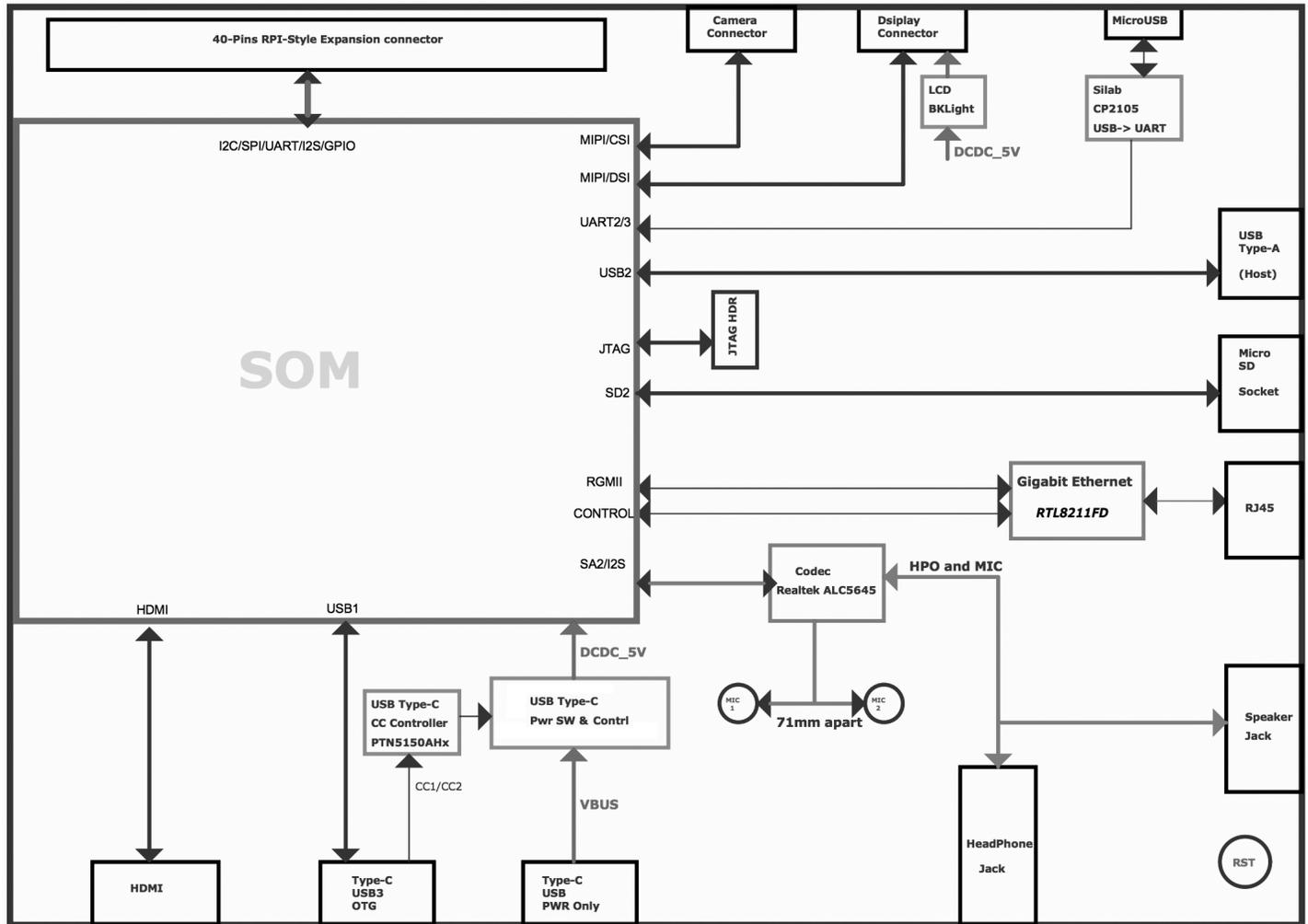
Figure 1. Block diagram of the baseboard components
