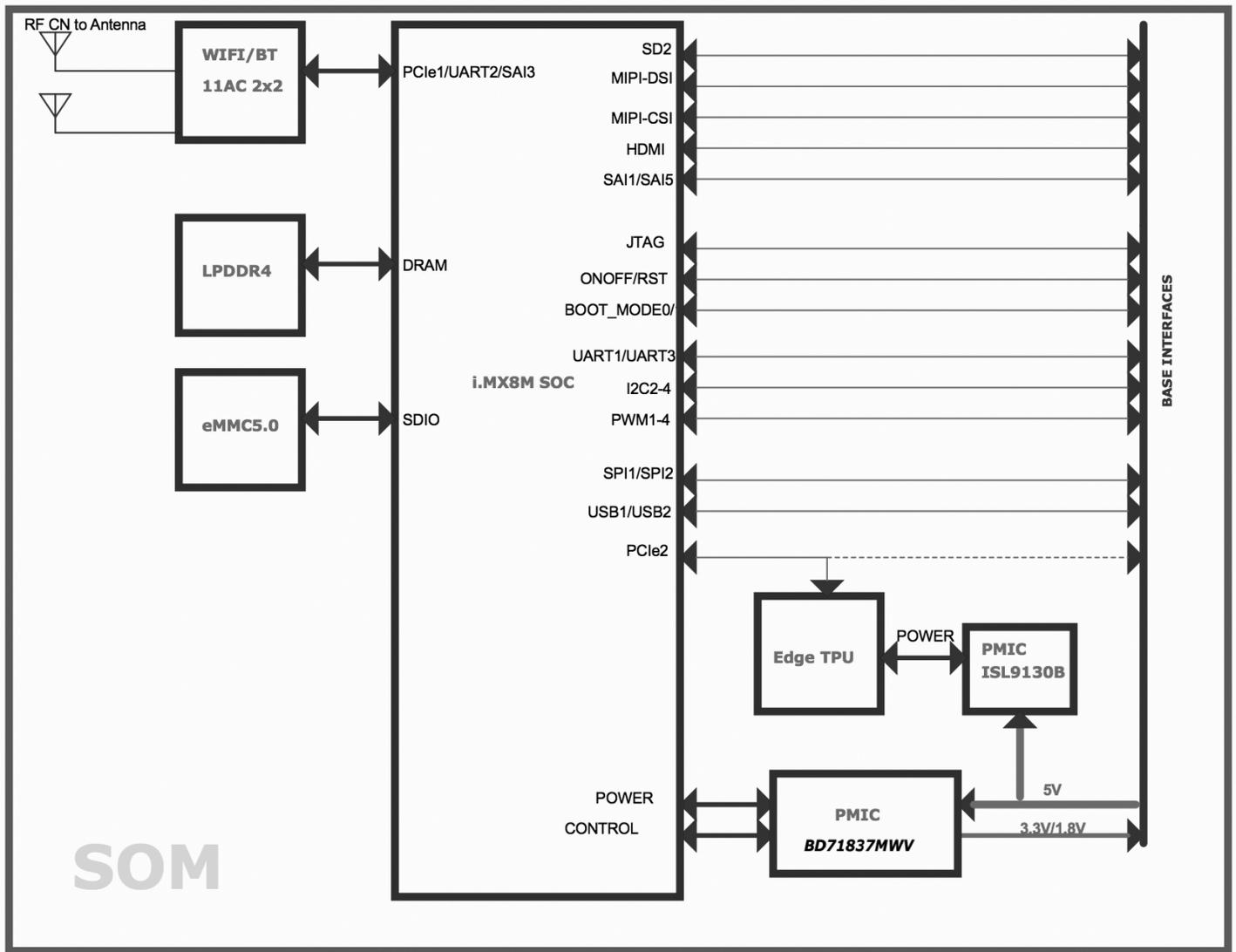
Figure 2. Block diagram of the SoM components
