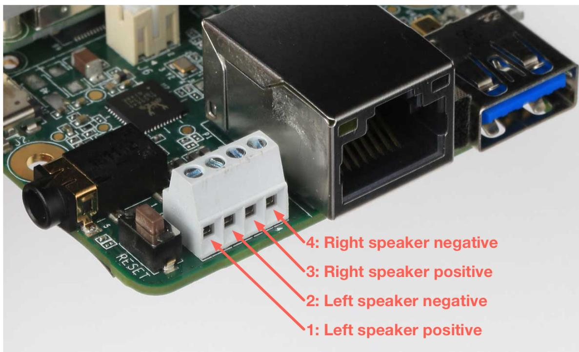
Figure 5. Stereo speaker terminals
