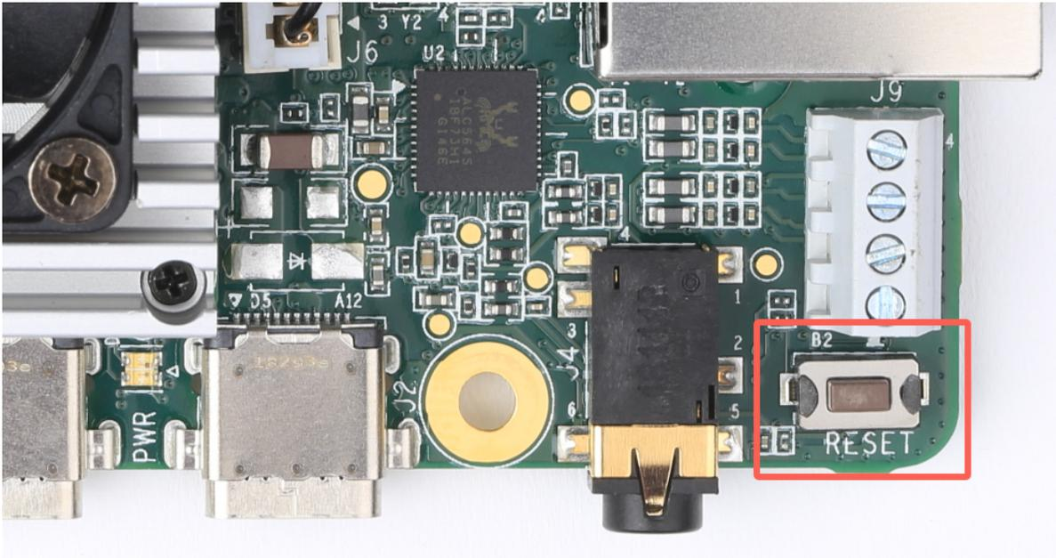
Figure 8. System reset button
