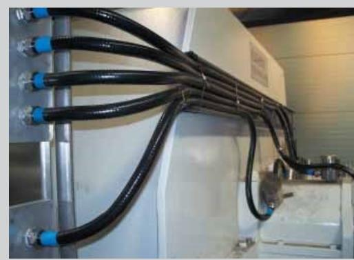
ring and insert are from PA6 (red for ISO metric, blue for Pg and white for NPT).
