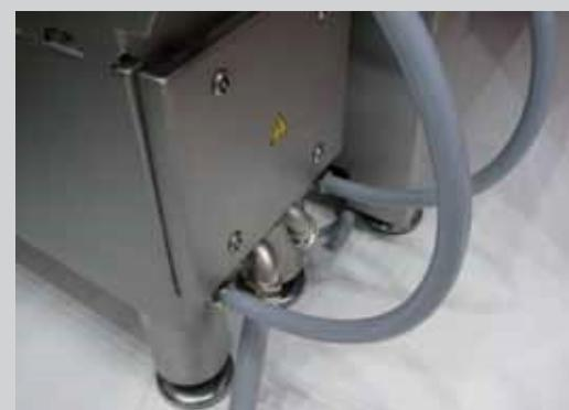
**Construction:** Stainless steel AISI-316 fitting, consisting of 4 parts (counter nut, clamping ring, ferrule and body).
