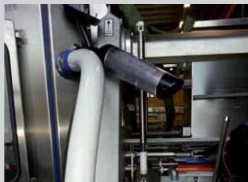
ring is from PA6. The blue rubber is made of TPE in accordance with FDA-CFR 21.
