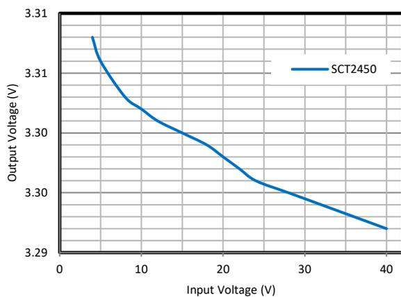
Figure 7. Line Regulation (Iout=5A)
