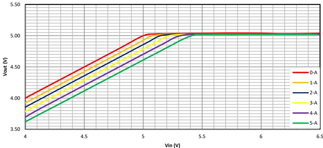
Figure 18. LDO Operation Characteristic ( Vout =5V )
