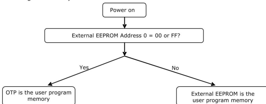
Once the user program development is completed using the external EEPROM then, the final program is ready to be written to the OTP. Then the external EEPROM is either removed physically or it is made inactive to the PS09 by writing the address 00 of the external EEPROM with 00 or FF. The following flowchart gives an overview of how the user program is developed using the EEPROM and transferred to the OTP finally.
