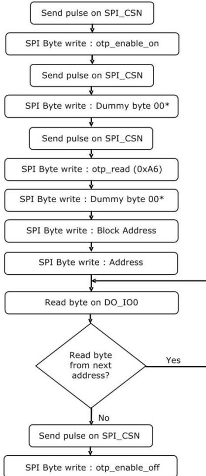
\* the Dummy byte (0x00) is required to be sent as it is needed because of timing purposes
