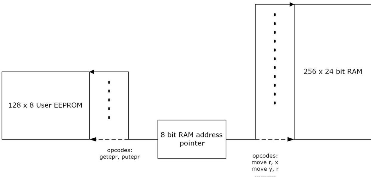
When the RAM address pointer is set to a value and op codes putepr and getepr are used, the RAM address pointer points to the respective byte in the user EEPROM. Hence operations are carried out with the respective user EEPROM byte. All other op codes like move r, x set the RAM address pointer to point to the RAM, hence the operation is performed in the RAM.
