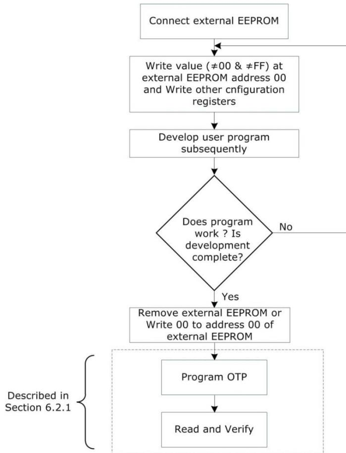
The PS09 Assembler Software which is used for user program development supports downloading the developed program to the external EEPROM or to the on chip OTP. The target for downloading the program can be selected from a drop down list on the Download page of the assembler.
