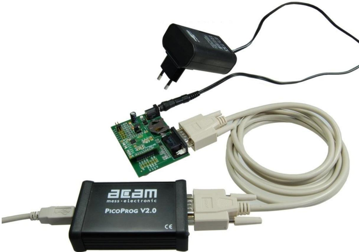
Figure 1-1: Components of the evaluation kit
