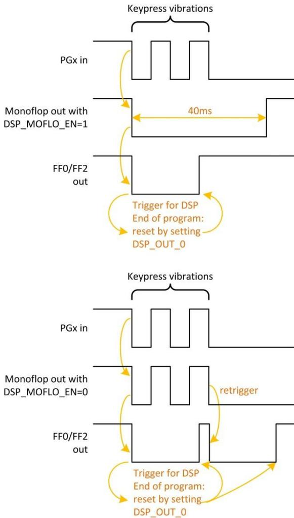
There is a possibility to activate a 40 ms debounce filter (“monoflop”) for the ports in case these are used as inputs. This might be useful especially in case the DSP is started by the pins (signals FF0, FF2). Figure 2-3 shows the effect of the monoflop filter.
