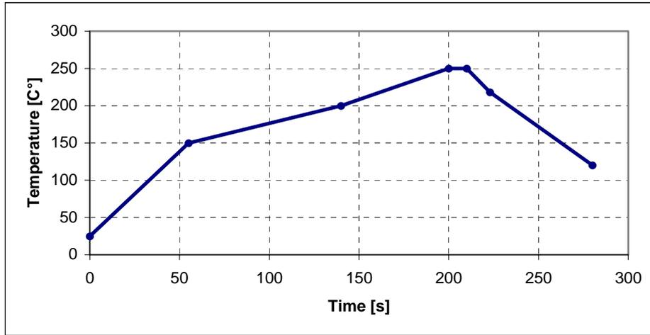
**Tolerance for Temperature settings T +0°C** (according to JEDEC J-STD-020C, July 2004)
