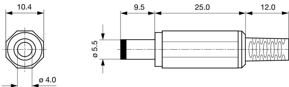
Cable diameter max. 4.0 mm
