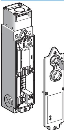
With the machine guard closed and locked, the resistance to forcible withdrawal of the actuator fitted to the guard is **Fzh 2300 N** according to the verification principle GS-ET19 ( $F_{zh} = F_{max}/1.3$ ).
