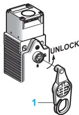
The manual unlocking of the guard using the tool 1 is useful in the following cases:
