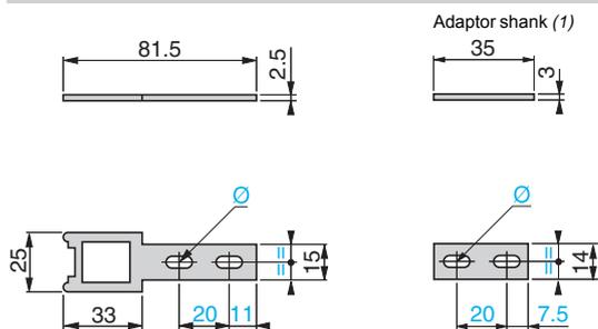
(1) Adaptor (included with actuator XCSZ01) for replacing, without drilling additional fixing hole, a guard switch XCK J with actuator ZCK Y07 by a guard switch XCSA, B, C or E with actuator XCSZ01.
