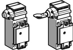
Metal key operated switches case for use on heavy machines **with low inertia** and operating in **arduous conditions** (shock or vibration exist), whereby the guard could open unintentionally. A key operated lock or a pushbutton enables the positive locking of the guard and its subsequent unlocking.
