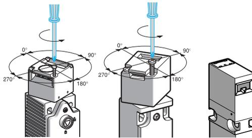
8 directions of actuation are possible for the actuator: 4 in the horizontal plane (1 for XCSMP), 4 from above the switch (1 for XCSMP), (4 alternative positions of the actuator slot, depending on the orientation of the head).
