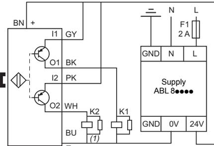
M12 connector (A coding) connection
