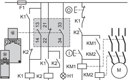
To activate K1, the lever or spindle must be rotated
