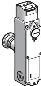
Safety interlock switches type XCSLF are available with a mushroom head pushbutton mounted on the rear of the switch for unlocking the machine guard whilst being held in the locked position by the solenoid. This manual unlocking using the mushroom head pushbutton for escape release is useful in the following cases:
