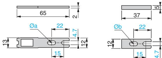
(1) Adaptor (included with actuator XCSZ11) for replacing, without drilling additional fixing hole, a key operated switch XCK T with actuator XCK Y01 by a key operated switch XCSTA with actuator XCSZ11.
