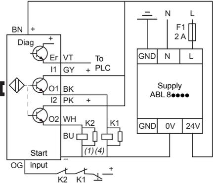
M12 connector (A coding) connection
