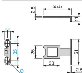
(1) Adaptor (included with actuator XCSZ01) for replacing, without drilling an additional fixing hole, a guard switch XCKJ or XCSL with actuator ZCKY07 with a guard switch XCSLF with actuator XCSZ01.
