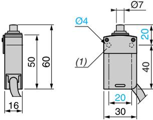
(1) Protective plate fixed by 5-lobe torque safety screws.
