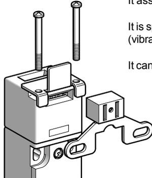
It assists in holding the guard closed by providing an extra retaining force of 5 daN.
