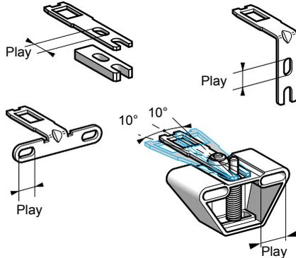
Their oblong fixing holes enable simple adjustment when mounting on moving guards.
