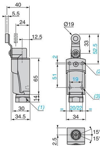
(1) Tapped entry for ISO M20 x 1.5 or Pg 13.5 cable gland or tapped 1/2" NPT.
