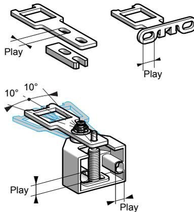
Their oblong fixing holes enable simple adjustment when mounting on moving guards.
