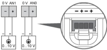
The (-) poles are connected internally.
