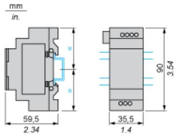
Screw Fixing (Retractable Lugs)
