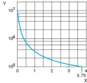
X Switching capacity (kVA)
