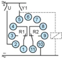
Function A : Power on Delay Relay
