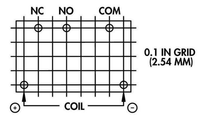
Connections and Wiring Diagrams
