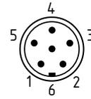
M8, 4-pole, with screw terminal or snap fitting      8 mm, 6-pole, with snap fitting
