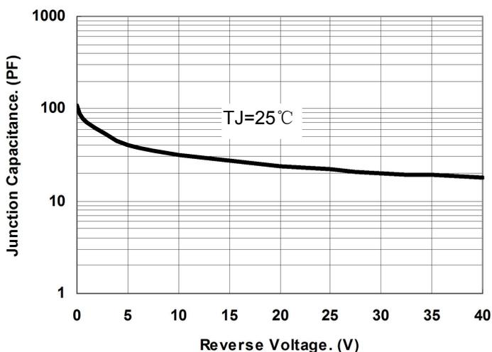
**Fig.1-Typical Junction Capacitance**
