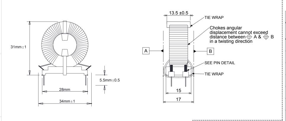
PRODUCT RANGE TYPE L(mH) I(Amps) R(mOhm) per winding CMV05 0.5 40 2300 CMV10 1.0 18 640 CMV20 2.0 7.5 160 CMV30 3.0 3.2 71 2.4 CMV40 4.0 40 CMV60 19 6.0 1.4 CMV80 8.0 0.74 9.6
