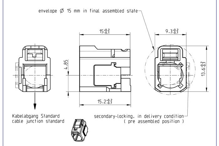
All dimensions are in mm; tolerances according to ISO 2768 m-H Y = Part number has to be accomplished by codification
