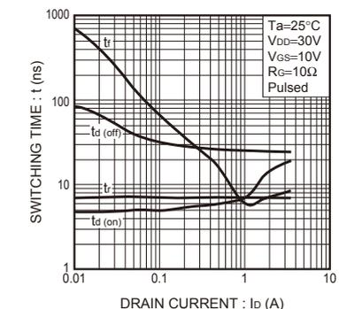
Fig.9 Switching Characteristics
