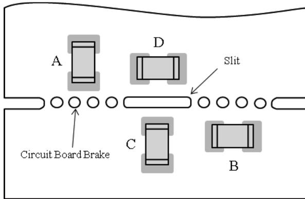
Stress strength according to the mounting position:
