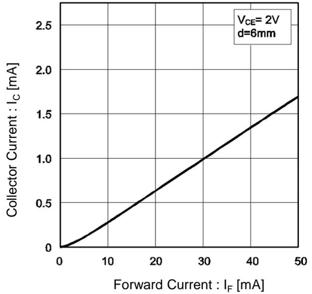
Fig.7 Output Characteristics
