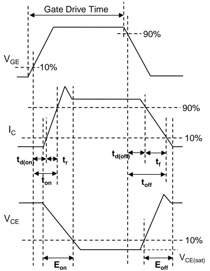
Fig.19 Inductive Load Waveform
