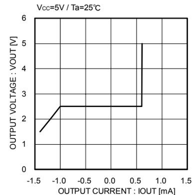
Fig.10 LPF operation amplifier output performance
