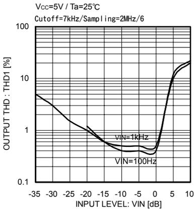
Fig.22 Input level vs distortion ratio characteristic 1
