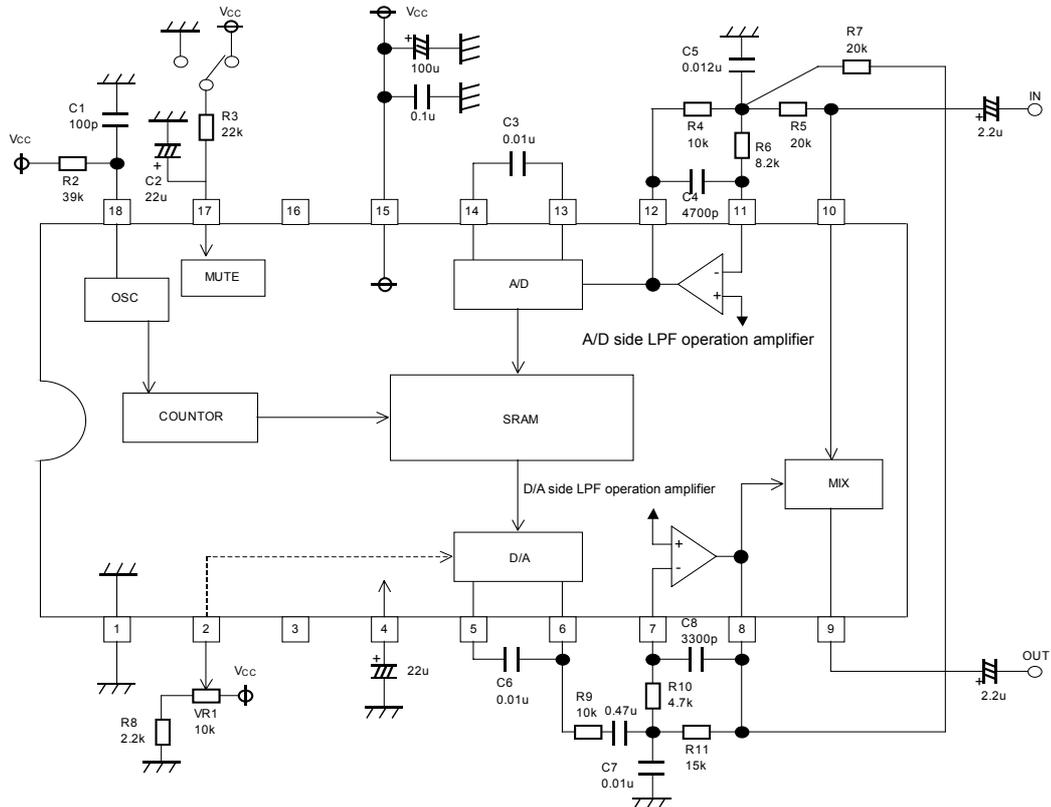
Fig.27 Application circuit
