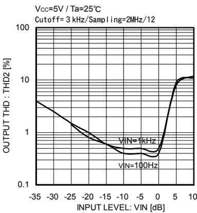
Fig.23 Input level vs distortion ratio characteristic 2
