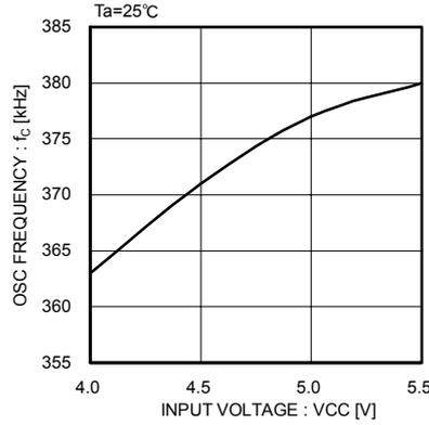
Fig.2 Oscillation frequency
