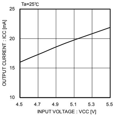
Fig.13 Circuit current
