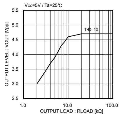
Fig.12 Delay side output load drive characteristic
