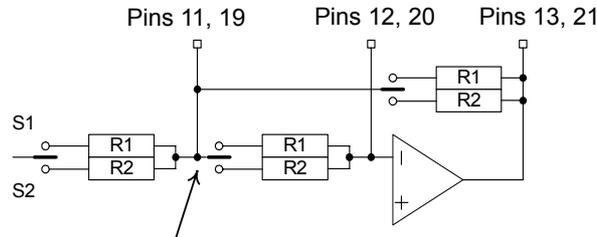
Note: In Pin 11, is an external capacity connection
