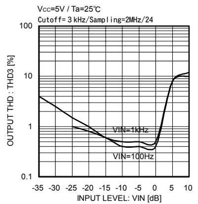
Fig.24 Input level vs distortion ratio characteristic 3
