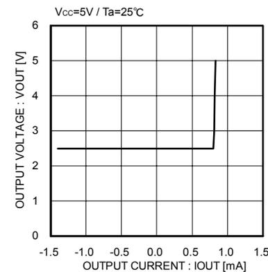
Fig.11 MIX operation amplifier output performance
