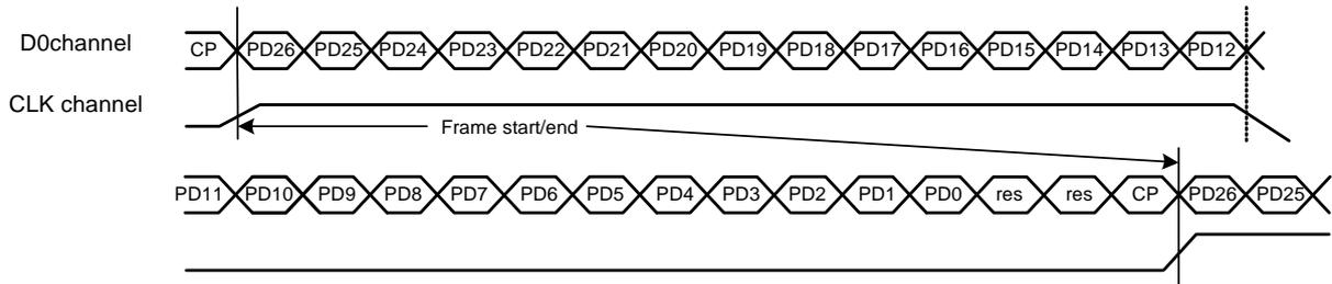
Fig.7. MSDL3 Protocol for 1-channel Data (27-bit)
