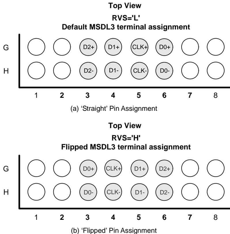
Fig.5. MSDL3 Pin Assignment
