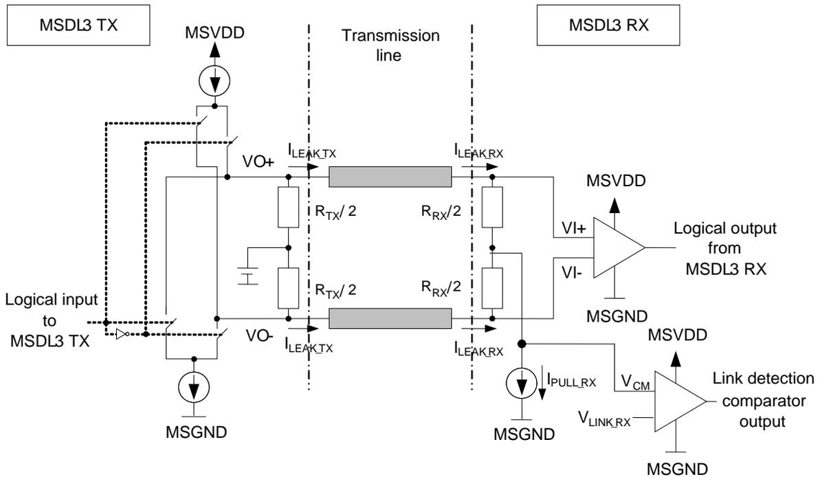
Fig.16. high-speed channel equivalent schematic.
