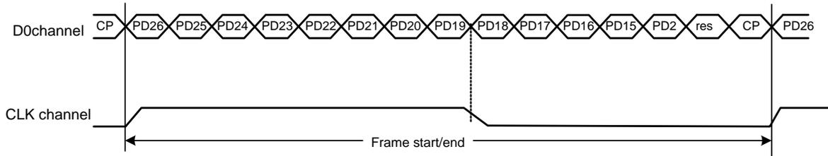
Fig.9. MSDL3 Protocol for 1-channel Data (13-bit)
