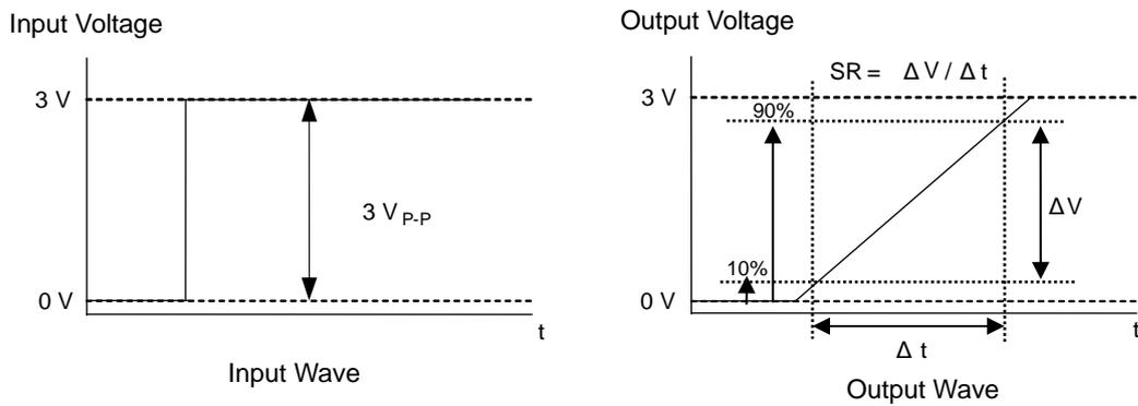
Figure 26. Slew Rate Input and Output Wave
