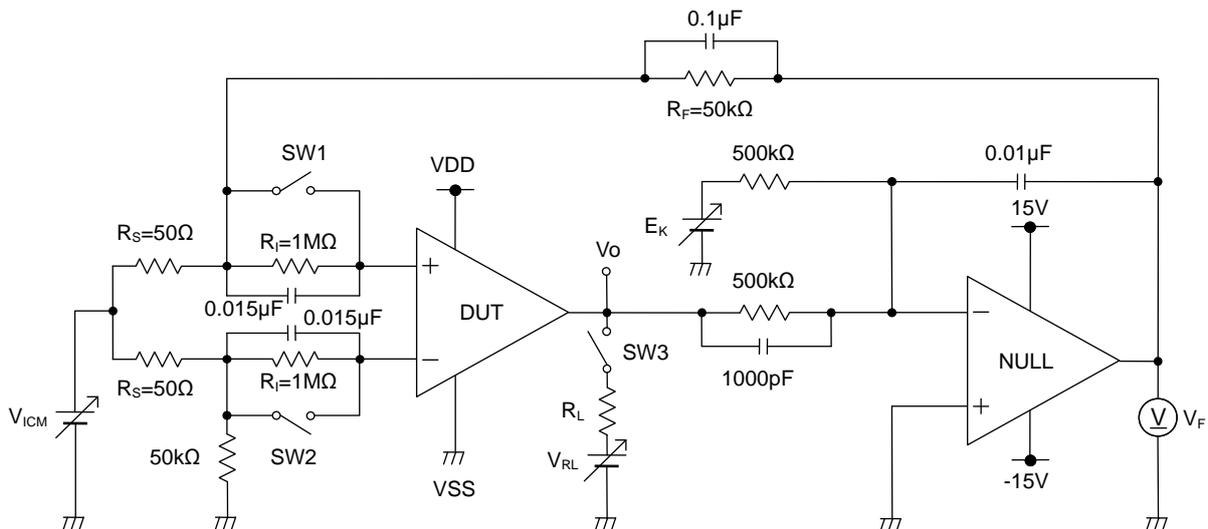
Figure 24. Test Circuit 1 (One Channel Only)
