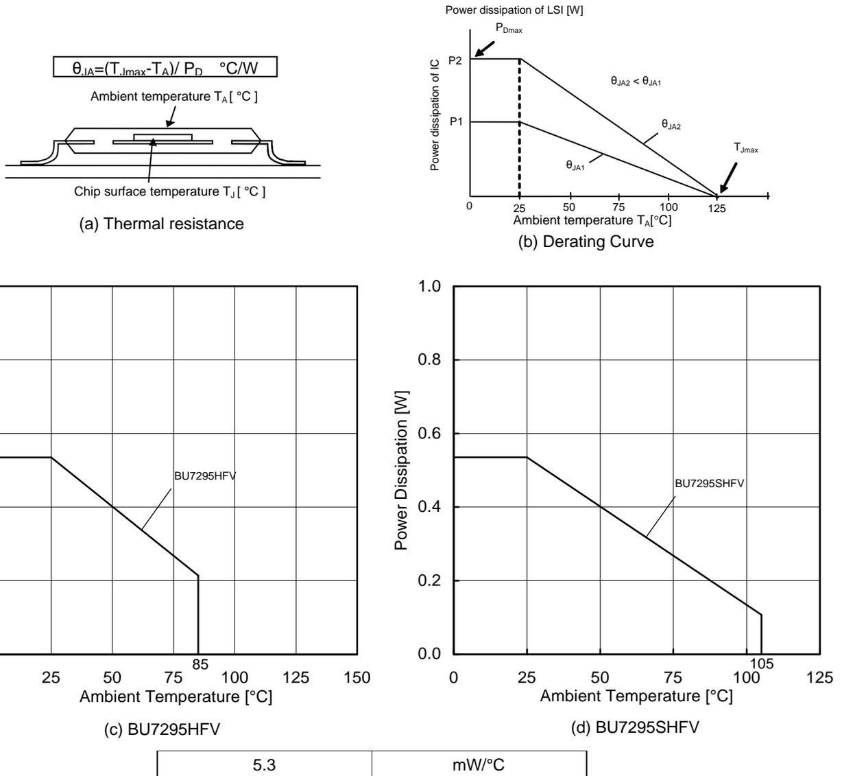
When using the unit above  $T_A=25^\circ\text{C}$ , subtract the value above per Celsius degree. Power dissipation is the value when FR4 glass epoxy board 70mm x 70mm x 1.6mm (copper foil area less than 3%) is mounted
