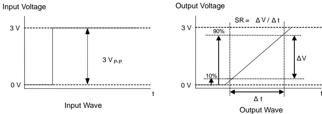
Figure 73. Slew Rate Input and Output Wave
