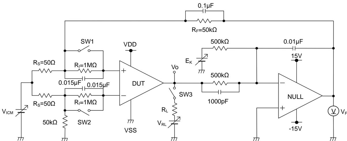
Figure 71. Test Circuit 1 (One Channel Only)
