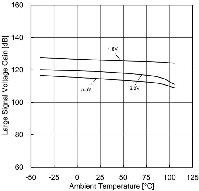
Figure 18. Large Signal Voltage Gain vs Ambient Temperature
