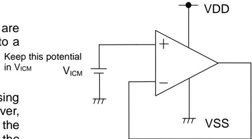
Figure 79. Example of Application Circuit for Unused Op-amp
