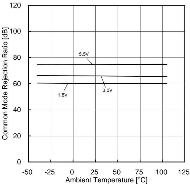
Figure 20. Common Mode Rejection Ratio vs Ambient Temperature
