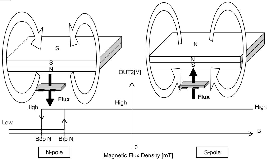
Figure 16. N-pole Detection
