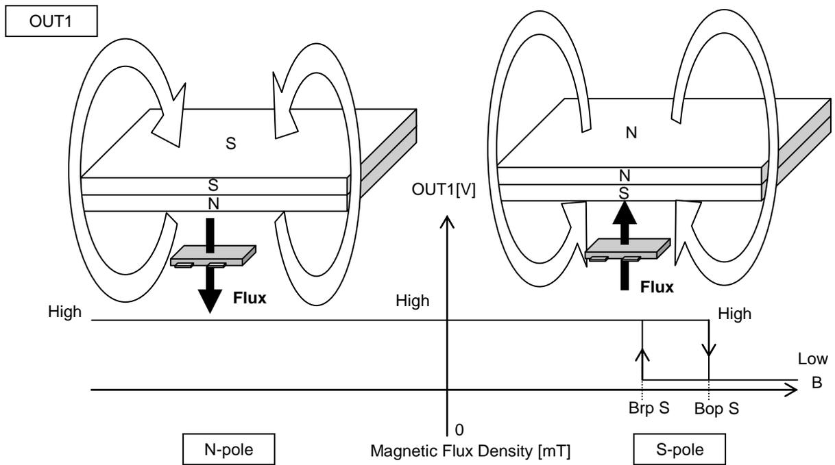
Figure 15. S-pole Detection
