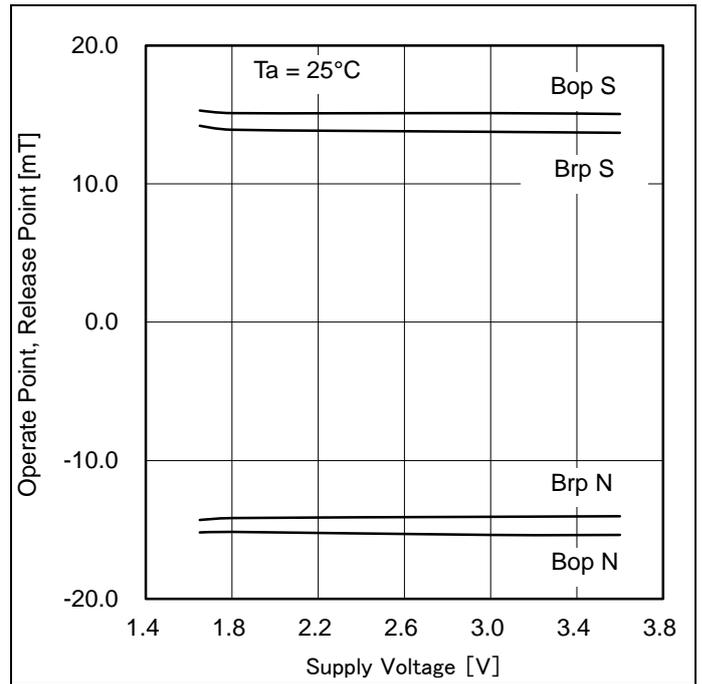
Figure 7. Operate Point, Release Point vs Supply Voltage
