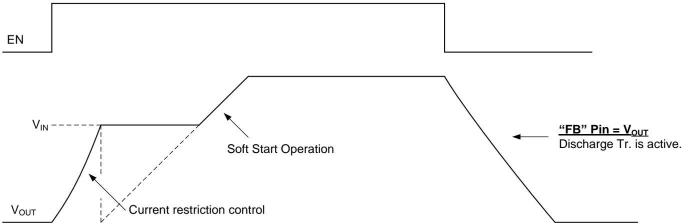
Figure 28. Start-up (Soft Start) and Shutdown Operation
