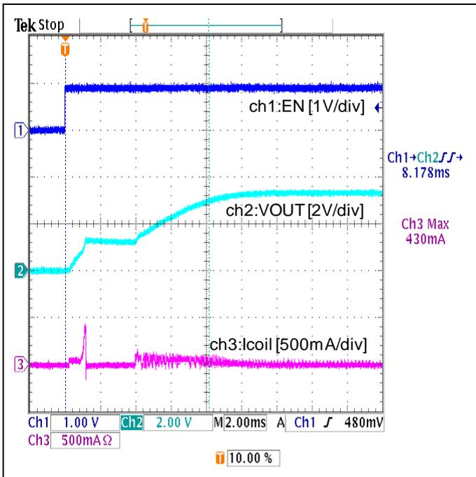
Figure 23. Start-up Waveform
