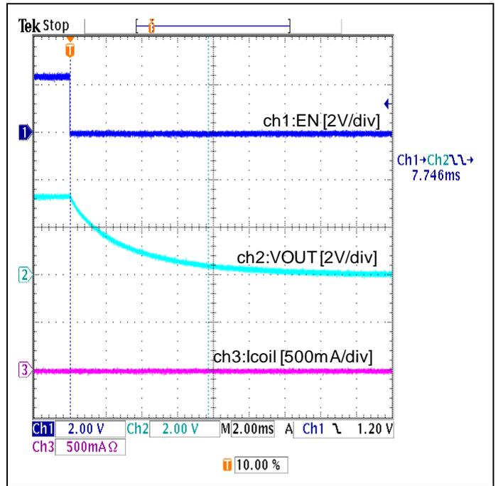
Figure 26. Shutdown Waveform
