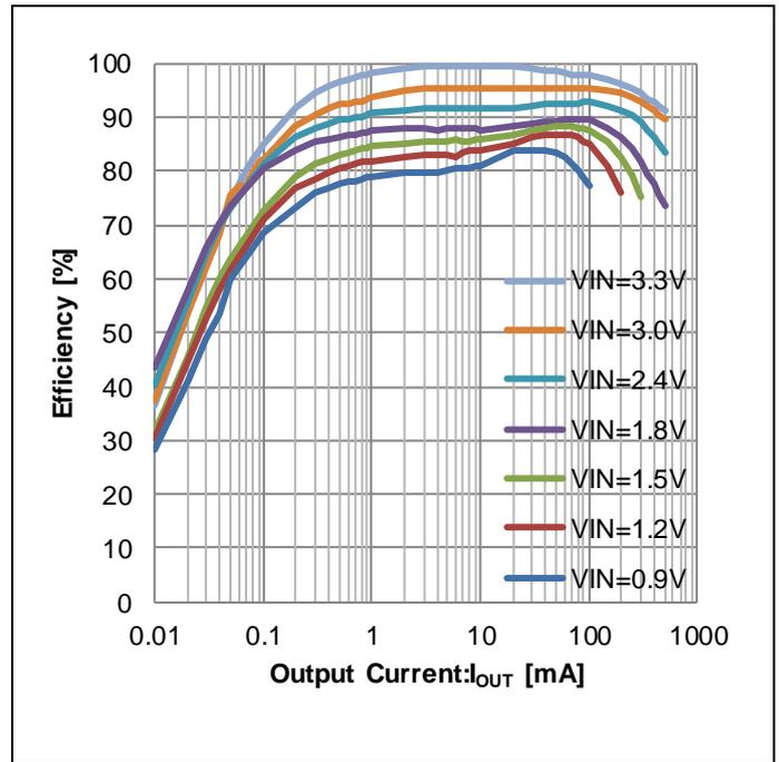
Figure 6. Efficiency vs Output Current (MODE=H: Auto-PFM/PWM)
