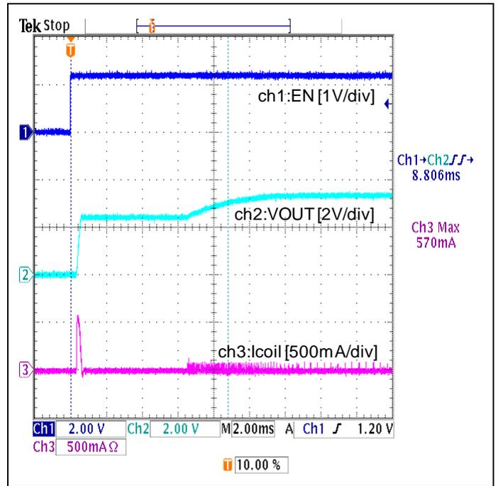
Figure 22. Start-up Waveform
