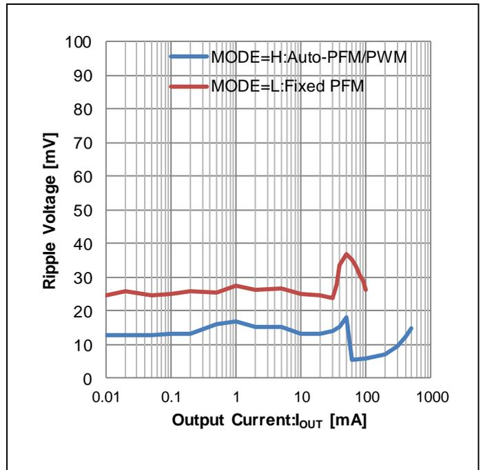
Figure 16. Ripple Voltage vs Output Current (VIN=2.4V)
