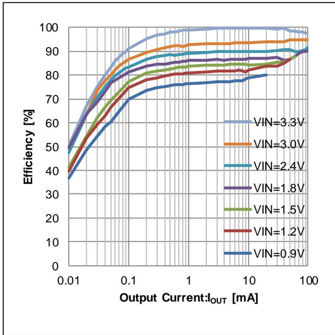
Figure 5. Efficiency vs Output Current (MODE=L: Fixed PFM)
