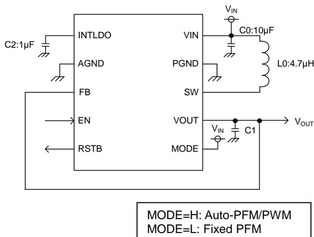
Figure 1. Application Circuit
