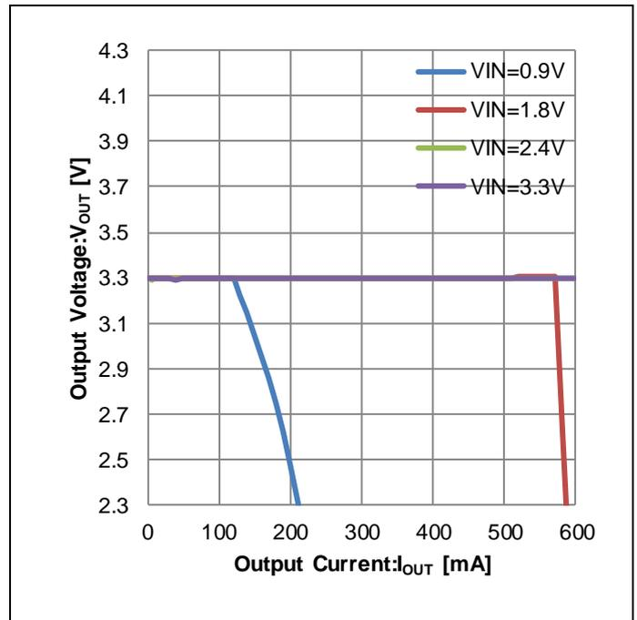
Figure 8. Output Voltage vs Output Current ("Load Regulation", MODE=H: Auto-PFM/PWM)
