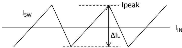
Figure 32. Switching Current
