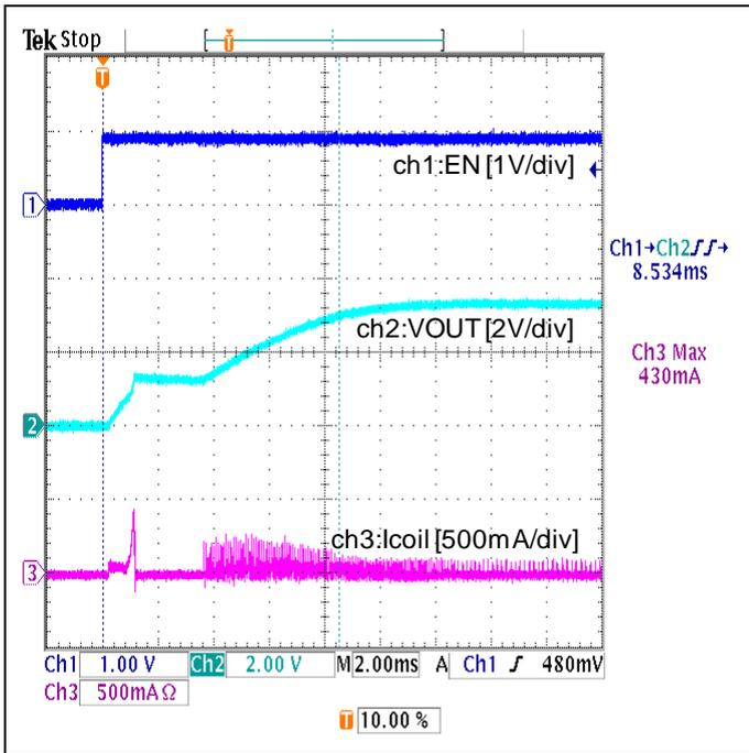
Figure 21. Start-up Waveform
