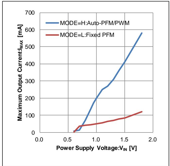
Figure 10. Maximum Output Current vs Power Supply Voltage
