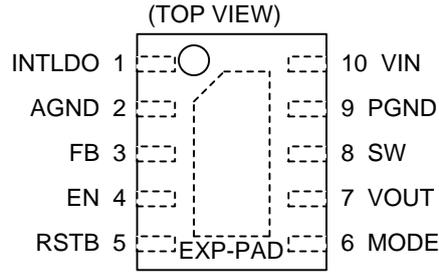
Figure 3. Pin Configuration
