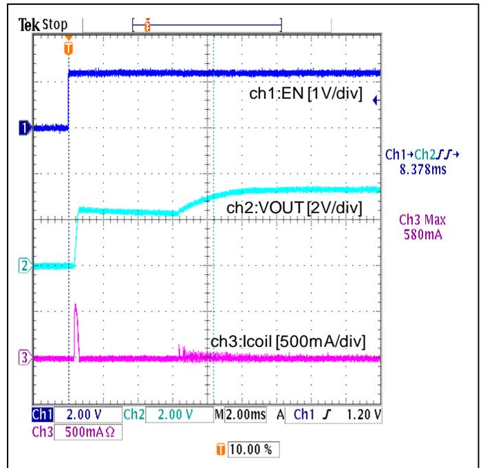
Figure 24. Start-up Waveform
