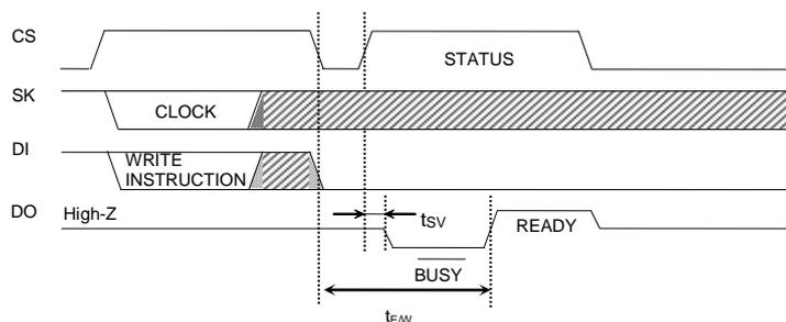
Figure 48.  $\overline{\text{READY}}$ / $\overline{\text{BUSY}}$  STATUS output timing chart
