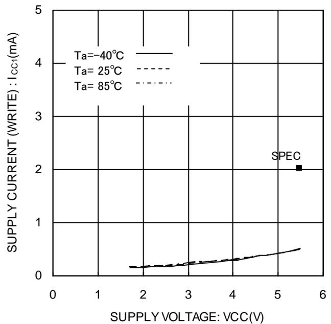
Figure 15. Supply current (WRITE)
