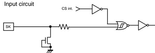
Figure 58. Input circuit (SK)
