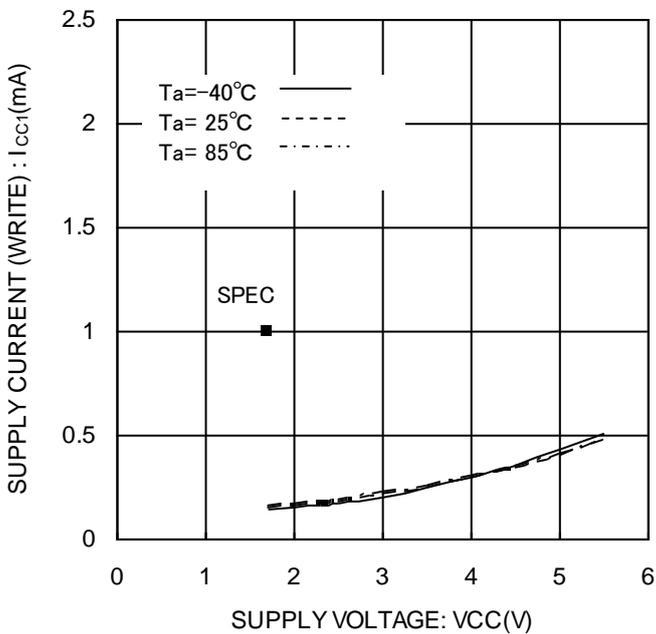
Figure 14. Supply current (WRITE)
