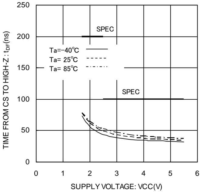
Figure 32. Time from CS to High-Z  $t_{Dr}$
