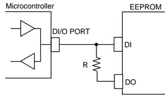
Figure 49. DI, DO control line common connection
