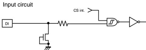
Figure 57. Input circuit (DI)
