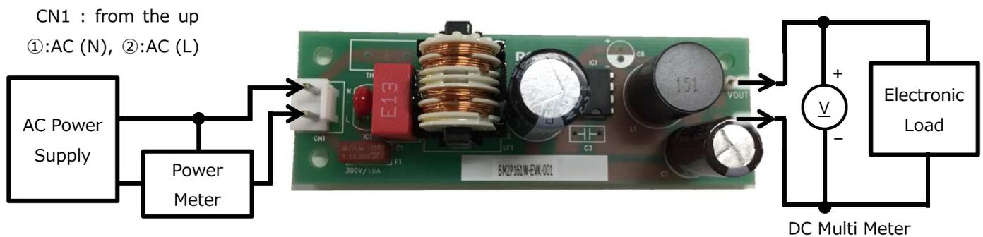
Figure 1. Connection Circuit
