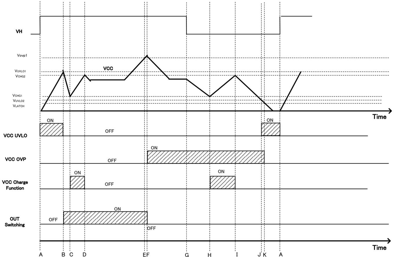
Figure 8. VCC UVLO / OVP Timing Chart
