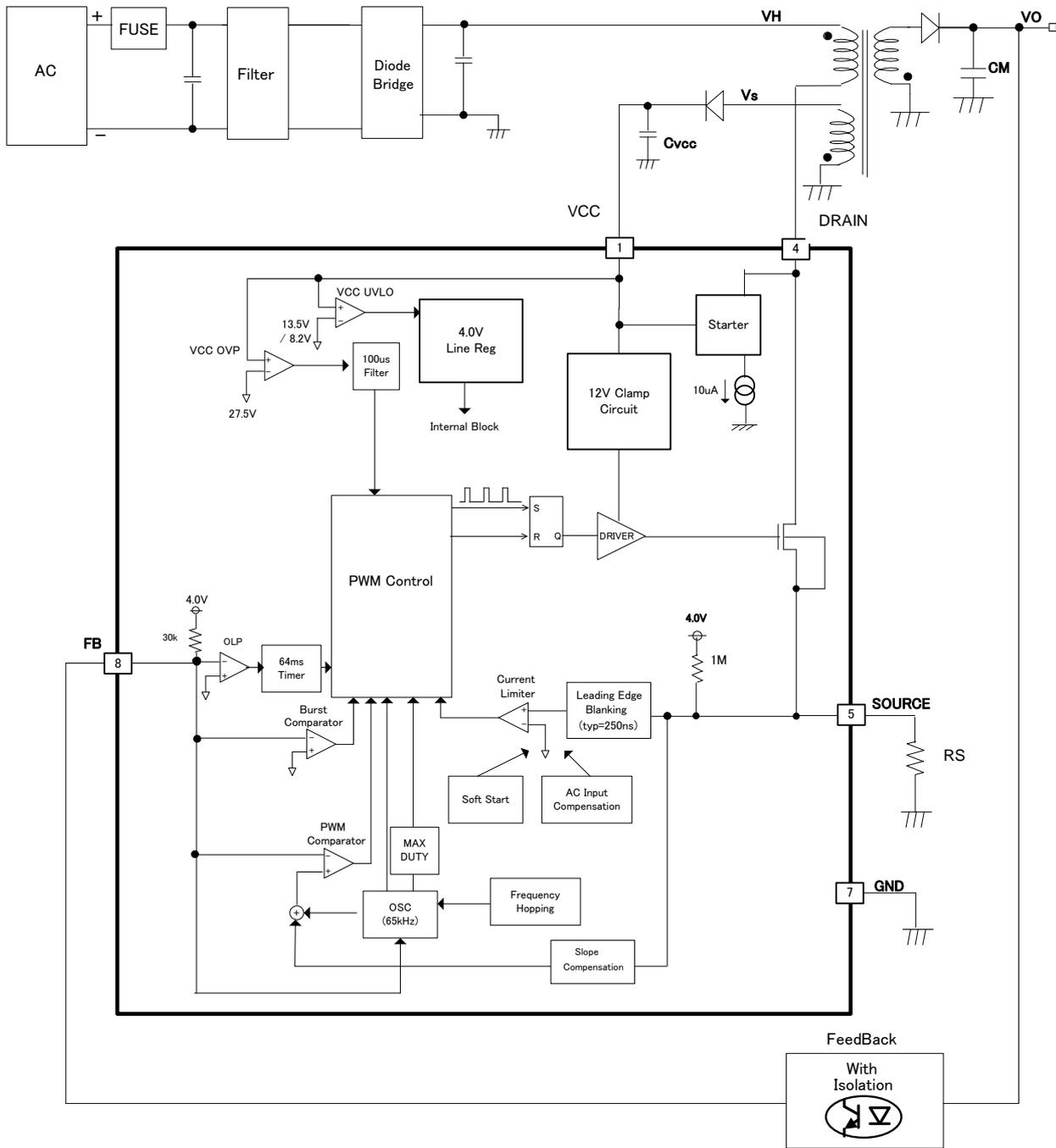
Figure 3. Block Diagram
