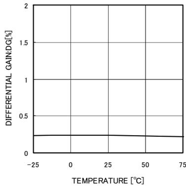
Fig.11 Differential Gain
