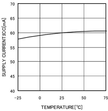
Fig.10 Circuit Current
