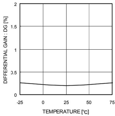
Fig.8 Differential Gain
