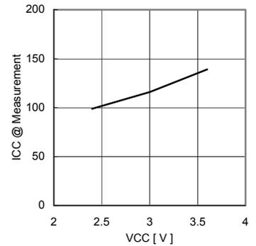
Fig.9  $V_{CC} - I_{CC}$  ( During measurement )
