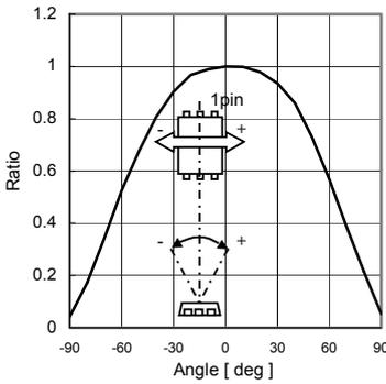
Fig.4 Directional Characteristics 1
