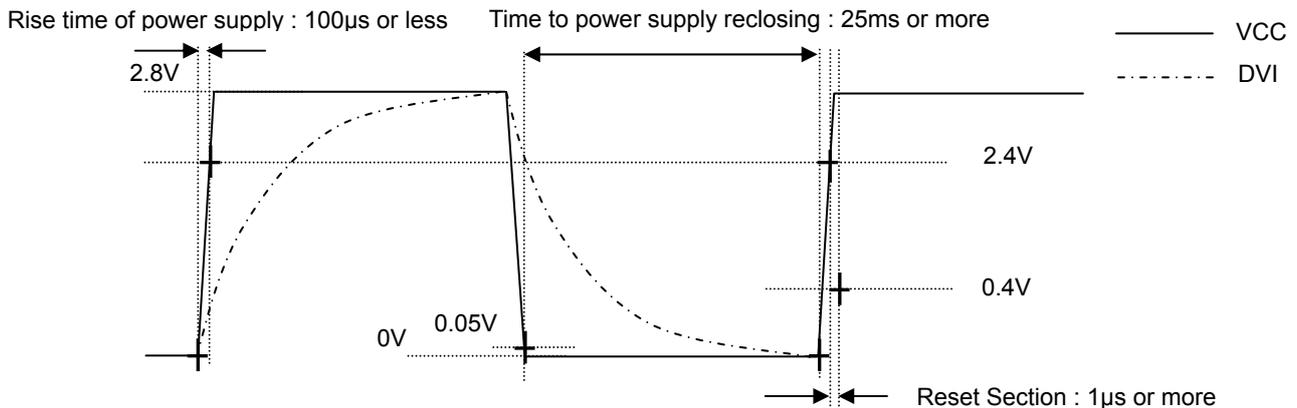
\* Please do the application design to secure Reset section 1µs or more after the reclosing of the power supply.
