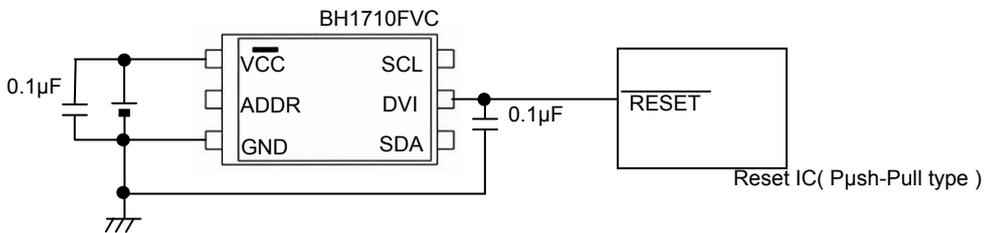
2, For Reset IC of the Open drain output
