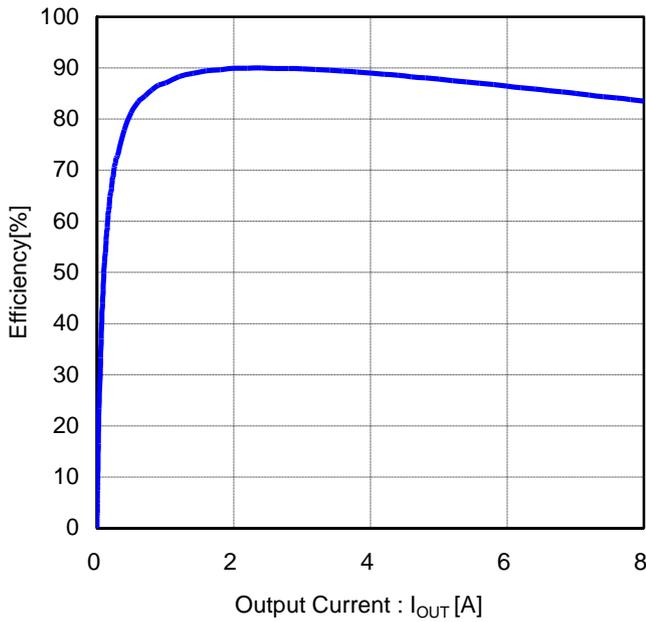
Figure 62. Efficiency vs Output Current
