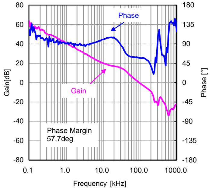
Figure 53. Loop Response  $I_{OUT}=8A$
