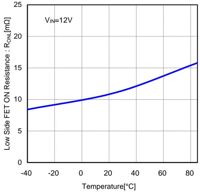
Figure 21. Low Side FET ON Resistance vs Temperature
