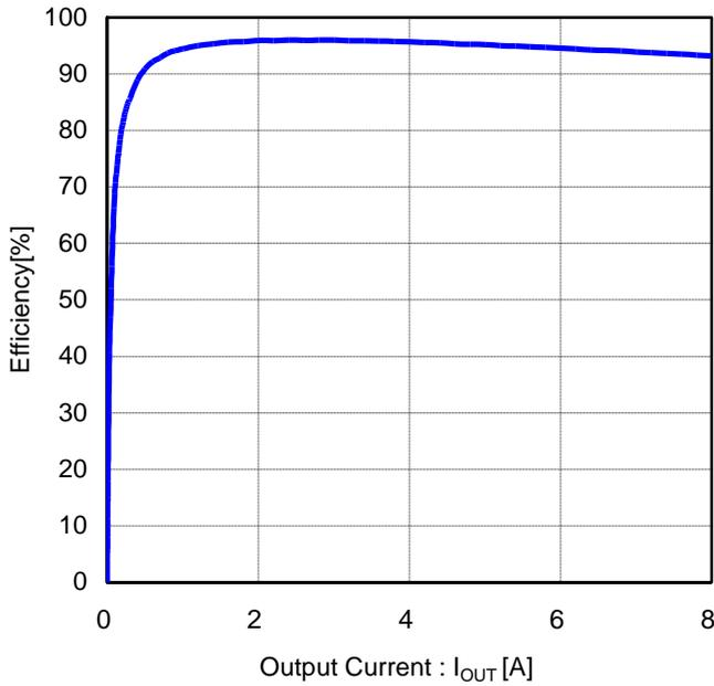
Figure 82. Efficiency vs Output Current
