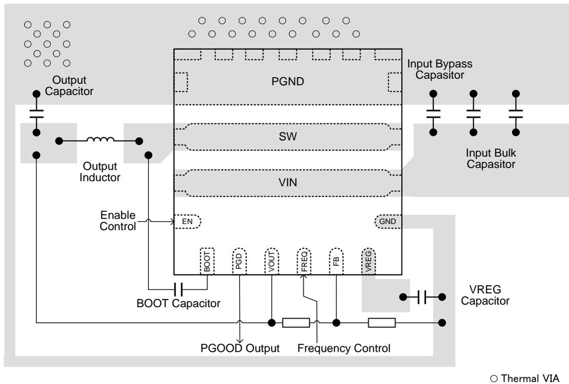
Figure 95. Example of PCB Layout (TOP VIEW)
