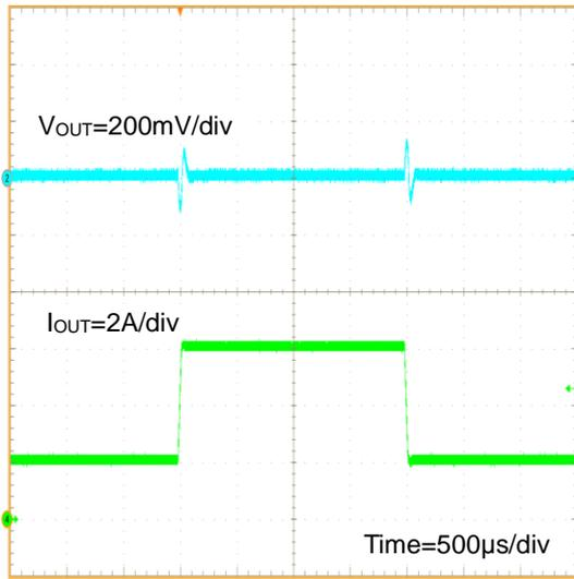
Figure 89. Load Transient Response  $I_{OUT}=2A - 6A$
