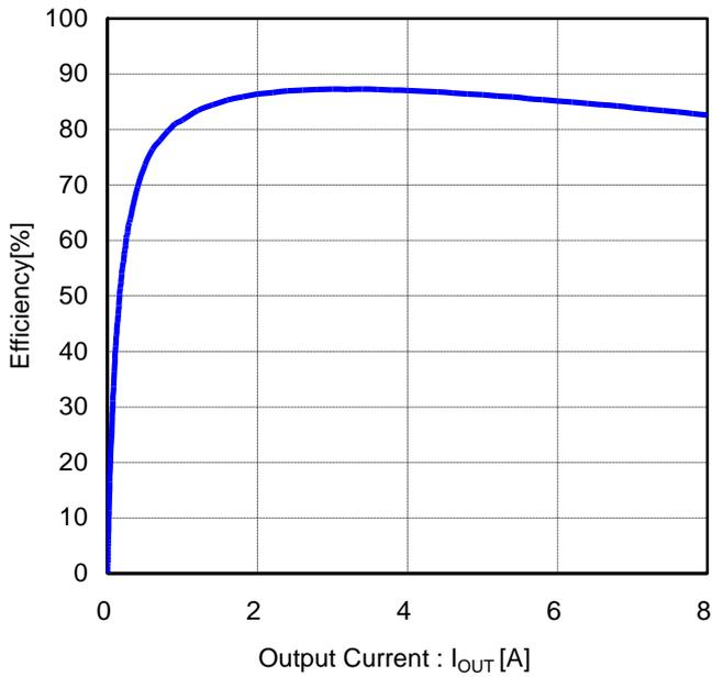
Figure 67. Efficiency vs Output Current ( $V_{IN}=12V$ ,  $V_{OUT}=1.2V$ ,  $FREQ=H(600kHz)$ )
