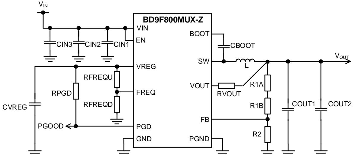
Figure 86. Application Circuit
