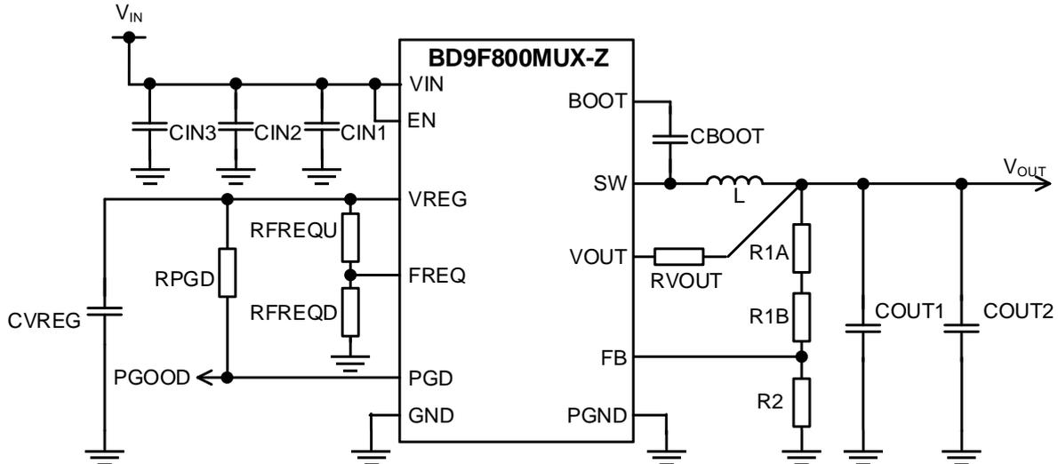
Figure 61. Application Circuit
