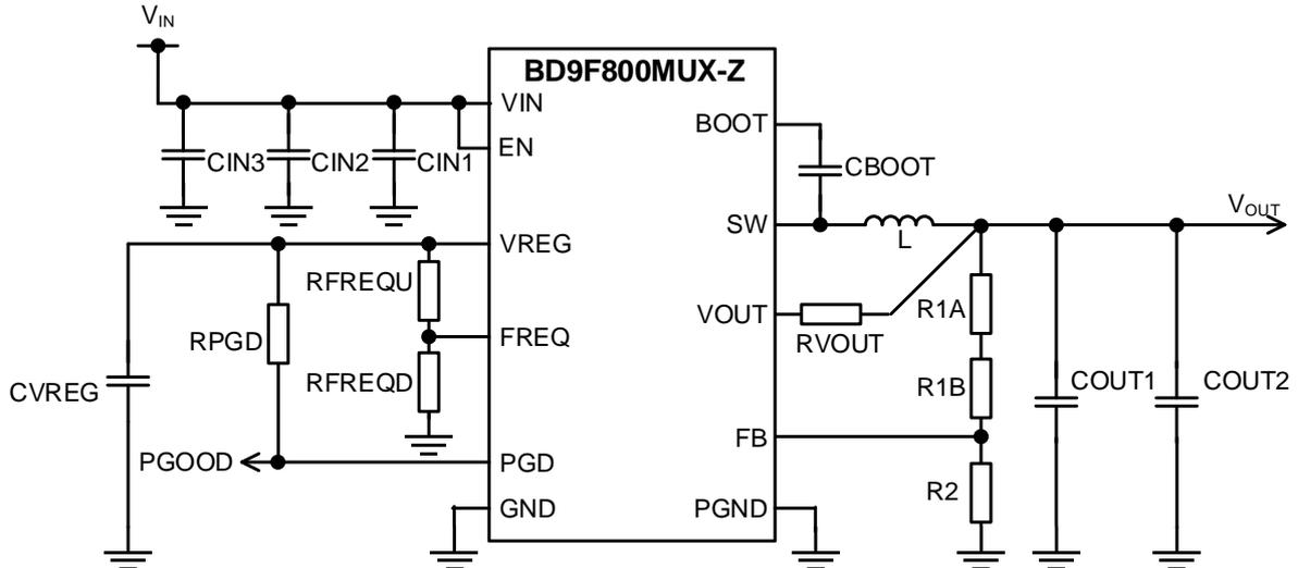
Figure 56. Application Circuit
