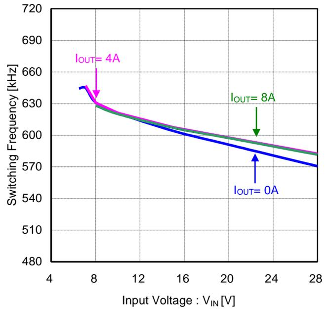
Figure 45. Switching Frequency vs Input Voltage (V<sub>OUT</sub>=5V, FREQ=H(600kHz))
