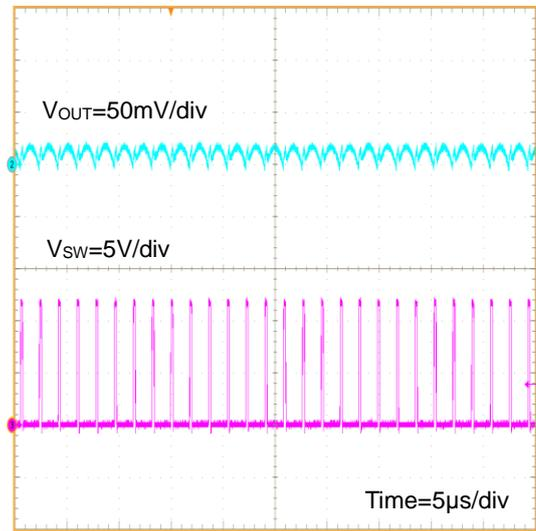
Figure 70.  $V_{OUT}$  Ripple  $I_{OUT}=8A$  ( $V_{IN}=12V$ ,  $V_{OUT}=1.2V$ ,  $FREQ=H(600kHz)$ )
