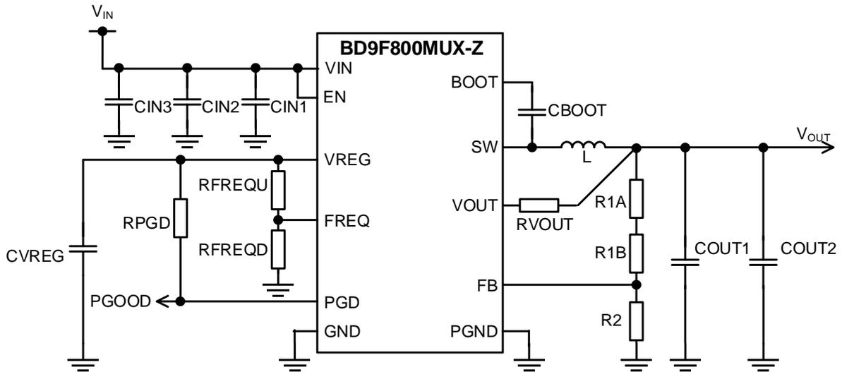
Figure 66. Application Circuit
