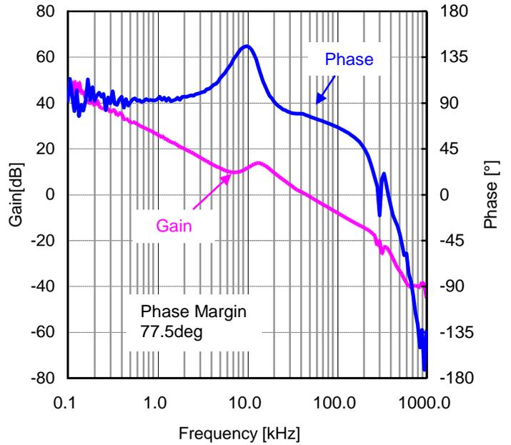
Figure 83. Loop Response  $I_{OUT}=8A$
