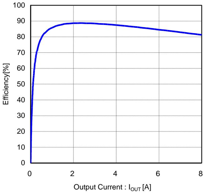
Figure 52. Efficiency vs Output Current
