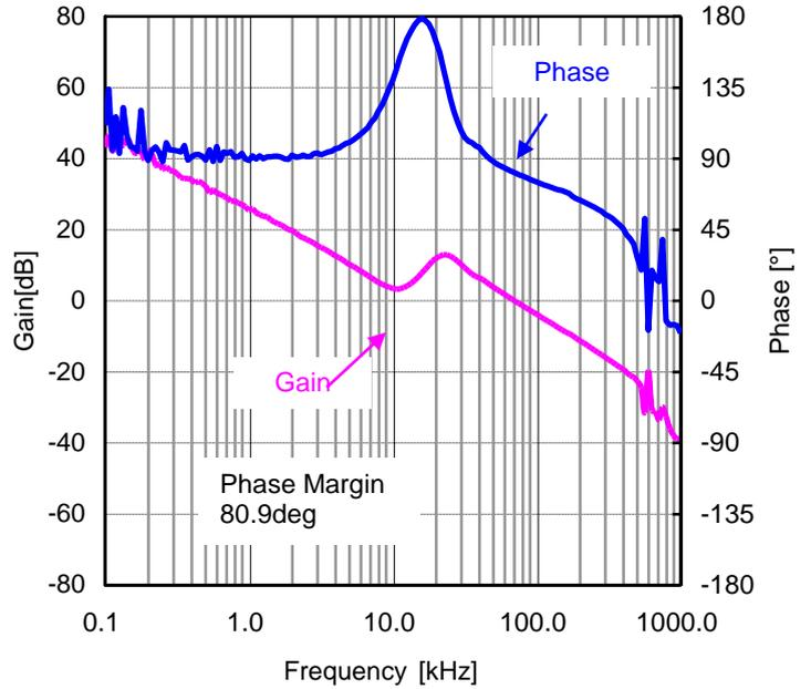
Figure 88. Loop Response  $I_{OUT}=8A$
