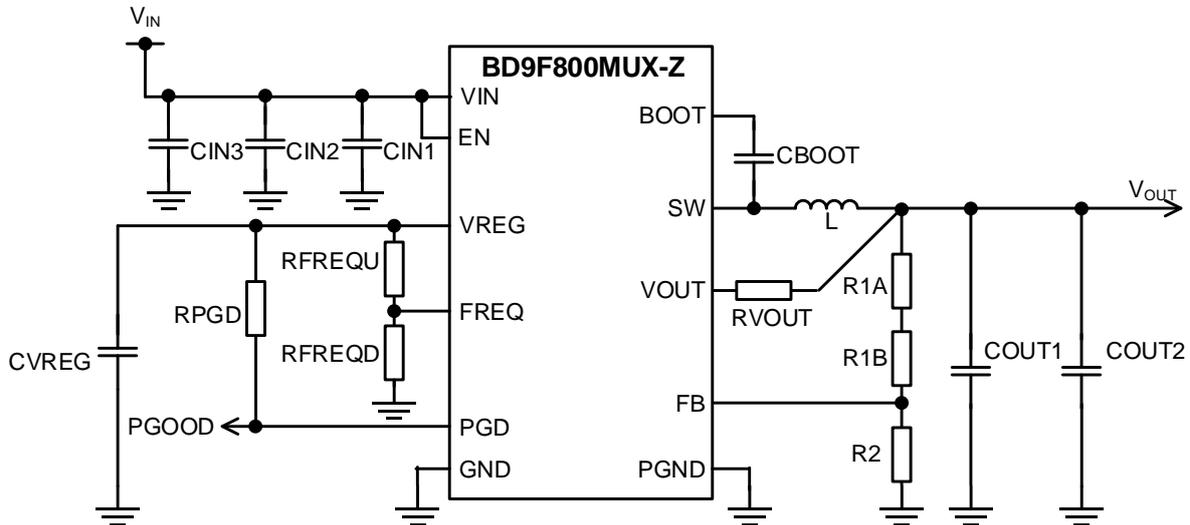
Figure 71. Application Circuit
