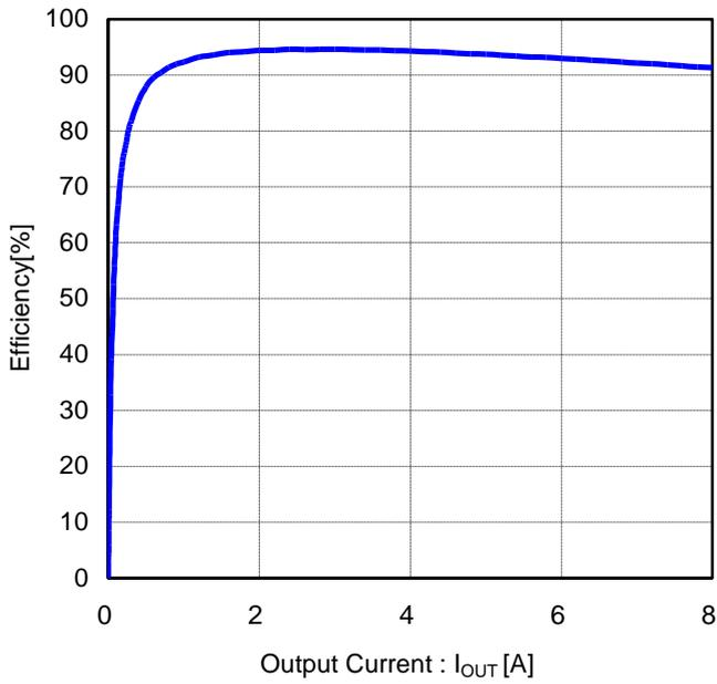
Figure 72. Efficiency vs Output Current
