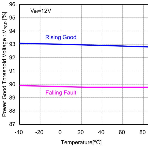
Figure 22. Power Good Threshold Voltage vs Temperature
