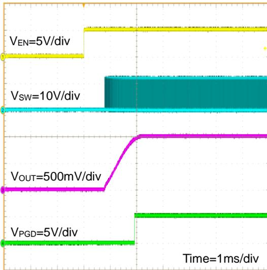
Figure 34. Start-up Waveform ( $V_{EN}=0V$  to  $5V$ )
