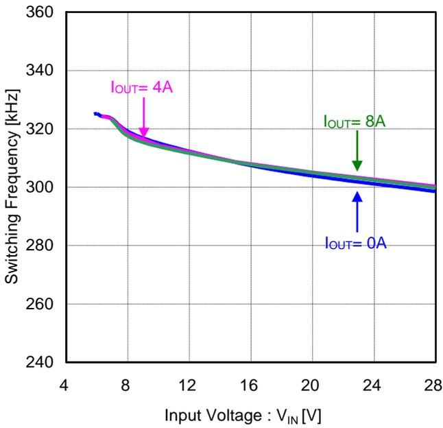
Figure 44. Switching Frequency vs Input Voltage (V<sub>OUT</sub>=5V, FREQ=L(300kHz))
