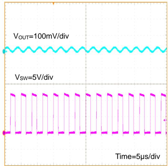
Figure 85.  $V_{OUT}$  Ripple  $I_{OUT}=8A$
