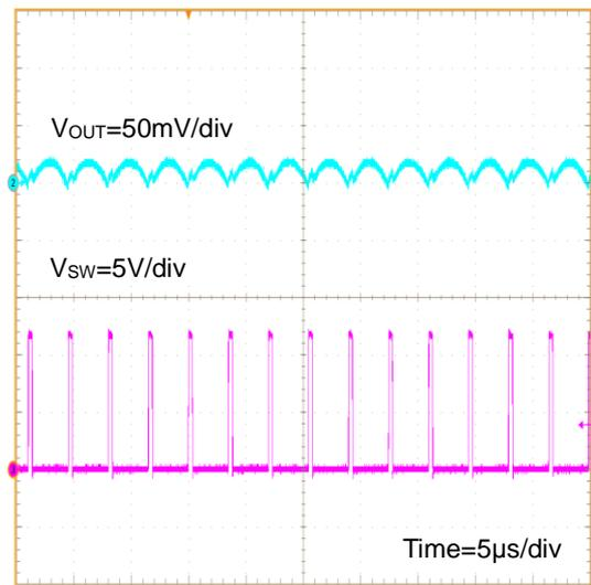
Figure 55.  $V_{OUT}$  Ripple  $I_{OUT}=8A$
