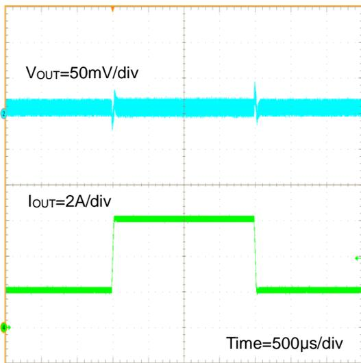
Figure 54. Load Transient Response  $I_{OUT}=2A - 6A$
