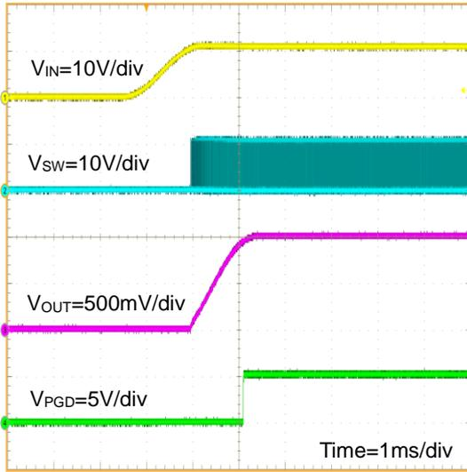
Figure 32. Start-up Waveform ( $V_{IN}=V_{EN}$ )
