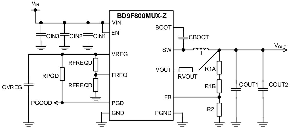
Figure 76. Application Circuit
