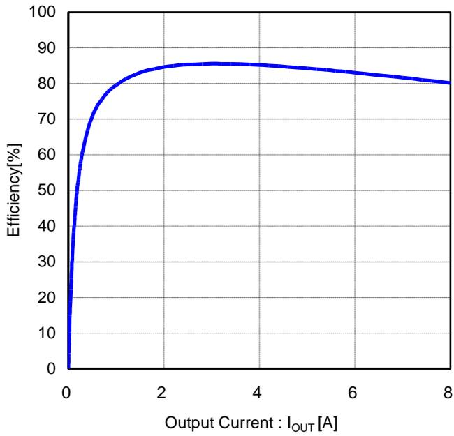
Figure 57. Efficiency vs Output Current (V<sub>IN</sub>=12V, V<sub>OUT</sub>=1V, FREQ=H(600kHz))
