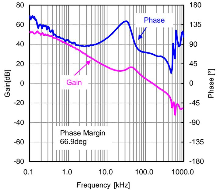
Figure 68. Loop Response  $I_{OUT}=8A$  ( $V_{IN}=12V$ ,  $V_{OUT}=1.2V$ ,  $FREQ=H(600kHz)$ )
