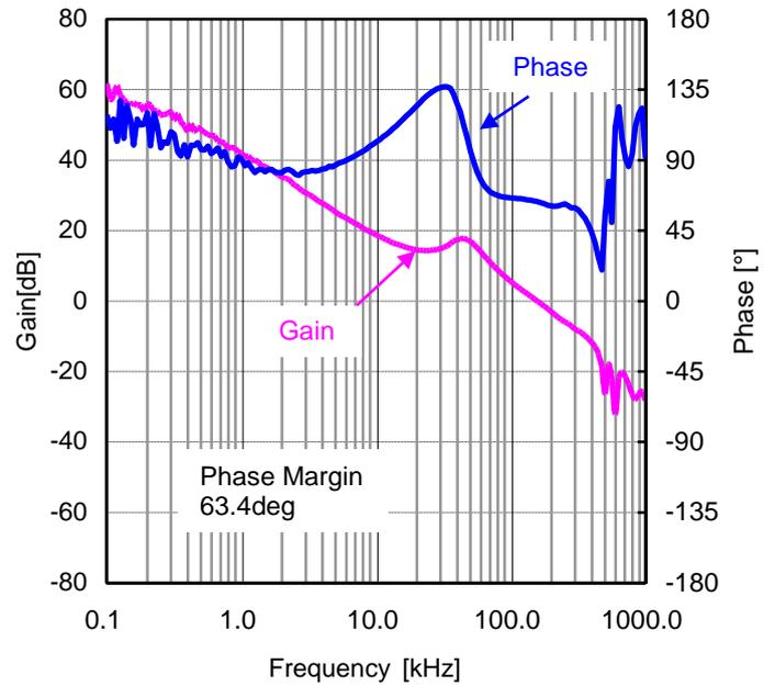
Figure 58. Loop Response I<sub>OUT</sub>=8A (V<sub>IN</sub>=12V, V<sub>OUT</sub>=1V, FREQ=H(600kHz))
