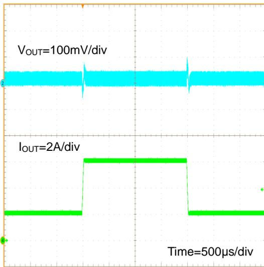
Figure 64. Load Transient Response  $I_{OUT}=2A - 6A$
