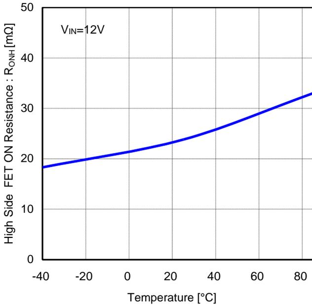
Figure 20. High Side FET ON Resistance vs Temperature
