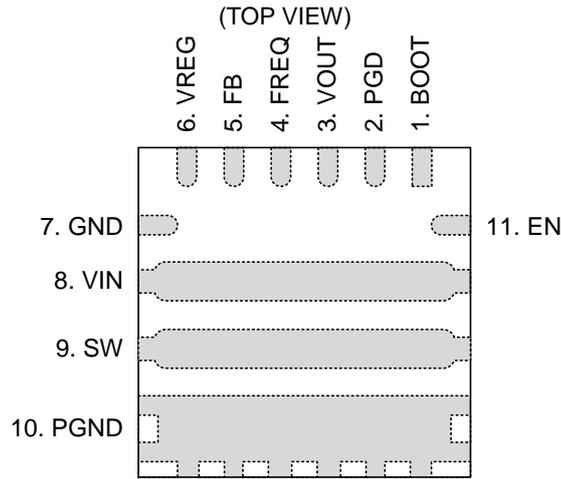
Figure 2. Pin Configuration
