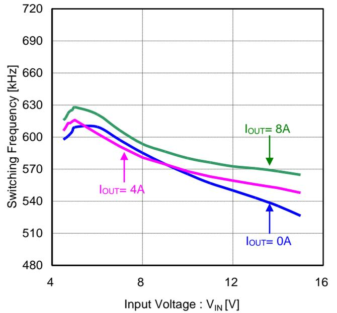
Figure 41. Switching Frequency vs Input Voltage (V<sub>OUT</sub>=1V, FREQ=H(600kHz))
