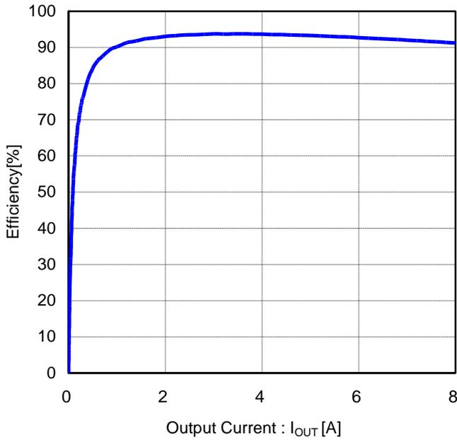
Figure 77. Efficiency vs Output Current ( $V_{IN}=12V, V_{OUT}=3.3V, FREQ=H(600kHz)$ )
