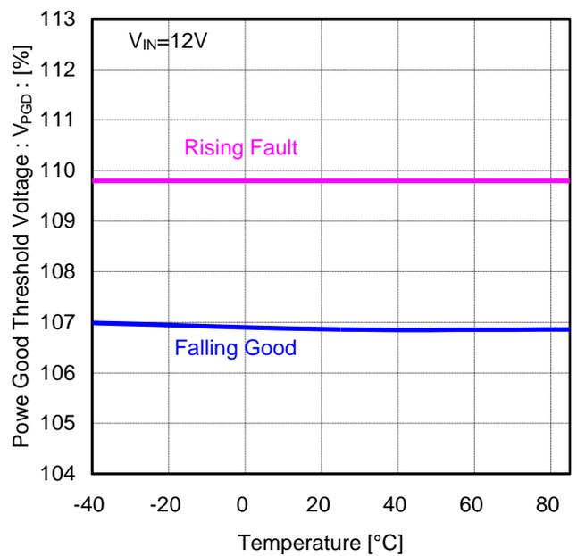
Figure 23. Power Good Threshold Voltage vs Temperature
