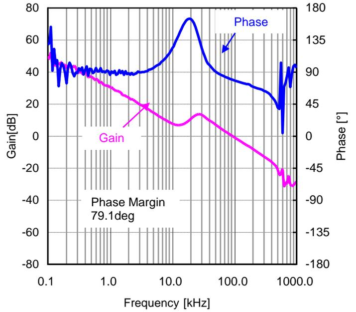
Figure 78. Loop Response  $I_{OUT}=8A$  ( $V_{IN}=12V, V_{OUT}=3.3V, FREQ=H(600kHz)$ )
