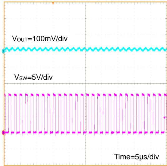
Figure 90.  $V_{OUT}$  Ripple  $I_{OUT}=8A$
