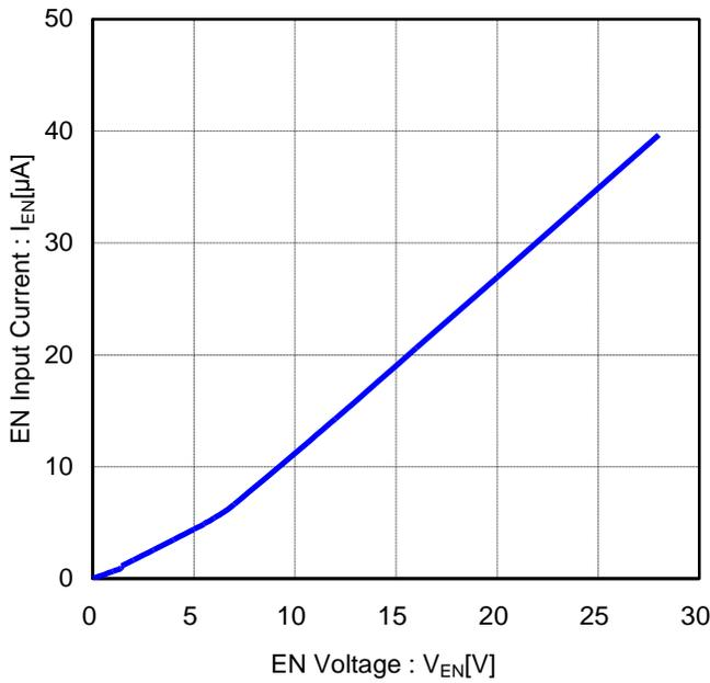
Figure 8. EN Input Current vs EN Voltage
