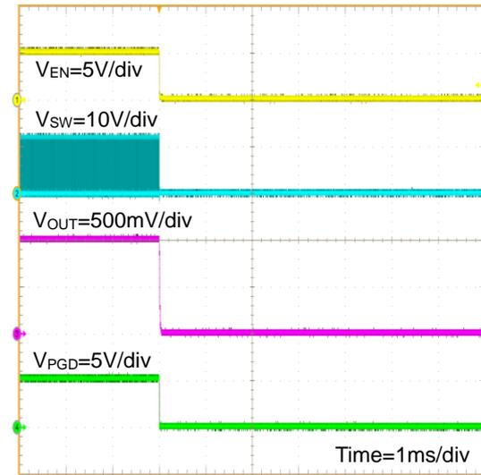
Figure 35. Shutdown Waveform ( $V_{EN}=5V$  to  $0V$ )
