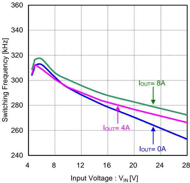
Figure 40. Switching Frequency vs Input Voltage (V<sub>OUT</sub>=1V, FREQ=L(300kHz))
