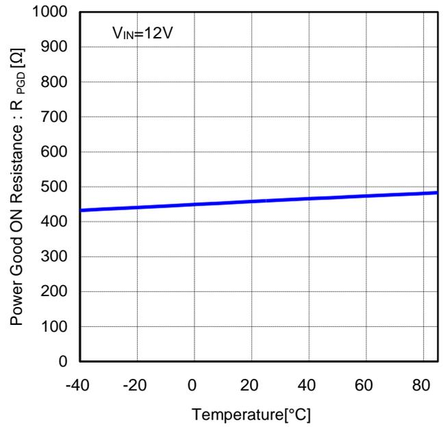
Figure 25. Power Good ON Resistance vs Temperature
