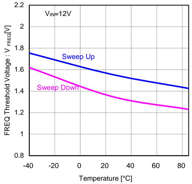
Figure 9. FREQ Threshold Voltage vs Temperature
