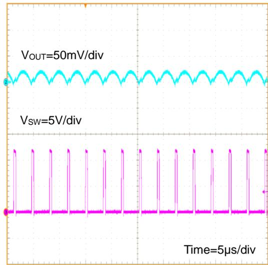
Figure 65.  $V_{OUT}$  Ripple  $I_{OUT}=8A$
