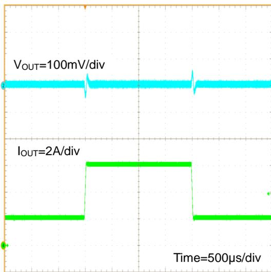
Figure 74. Load Transient Response IOUT=2A - 6A
