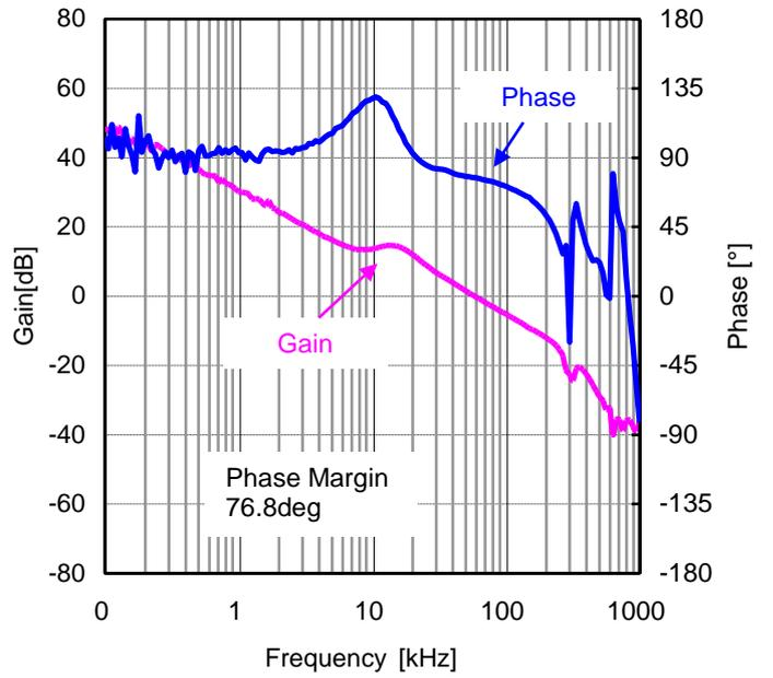
Figure 73. Loop Response IOUT=8A
