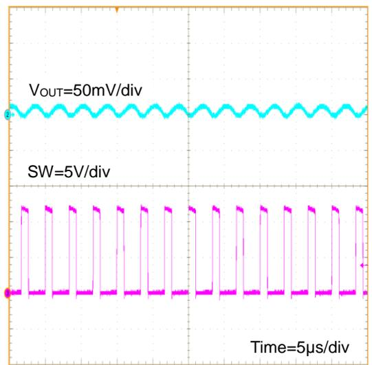
Figure 75. VOUT Ripple IOUT=8A
