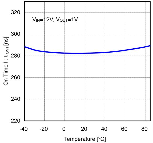
Figure 17. On Time 1 vs Temperature
