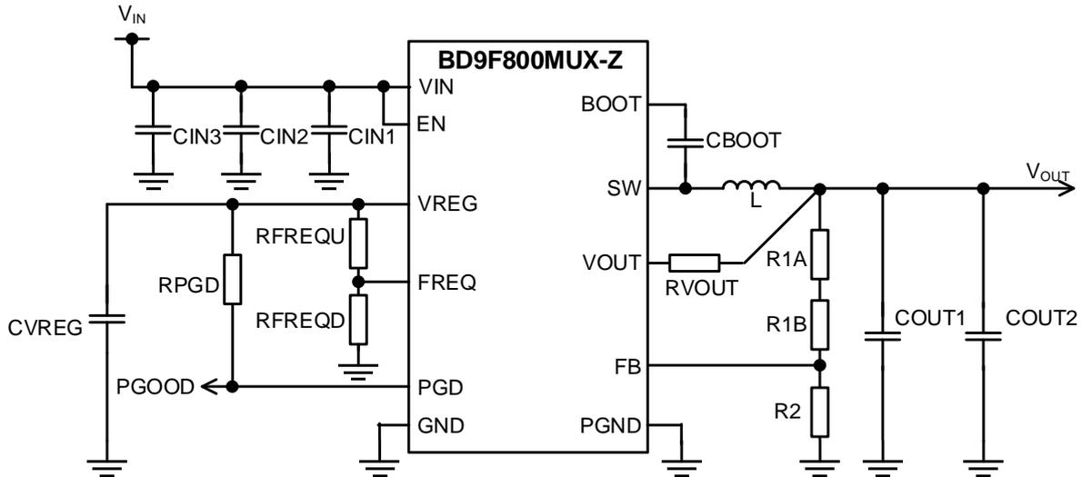
Figure 51. Application Circuit
