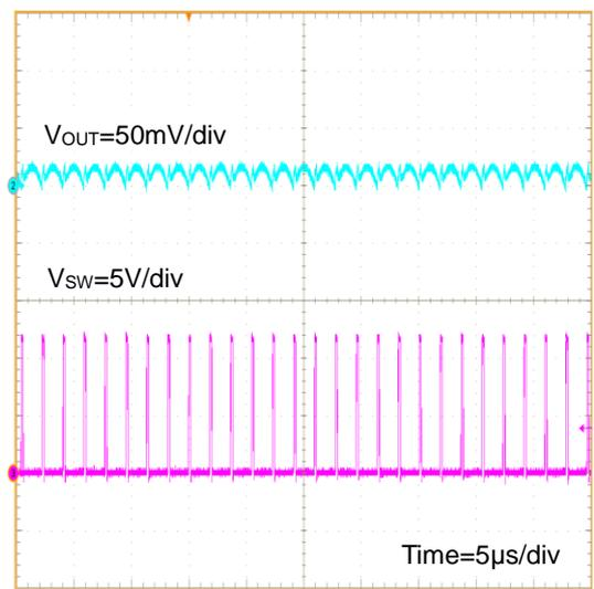
Figure 60. V<sub>OUT</sub> Ripple I<sub>OUT</sub>=8A (V<sub>IN</sub>=12V, V<sub>OUT</sub>=1V, FREQ=H(600kHz))
