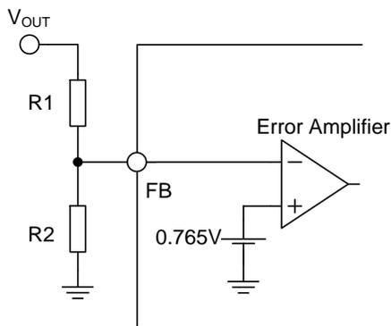
Figure 93. Feedback Resistor Circuit
