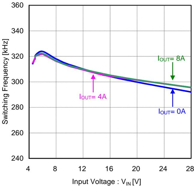
Figure 42. Switching Frequency vs Input Voltage (V<sub>OUT</sub>=3.3V, FREQ=L(300kHz))
