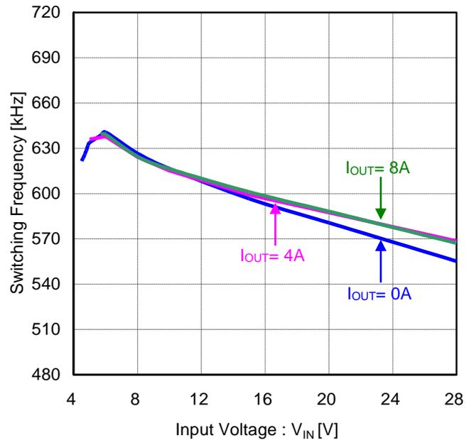
Figure 43. Switching Frequency vs Input Voltage (V<sub>OUT</sub>=3.3V, FREQ=H(600kHz))
