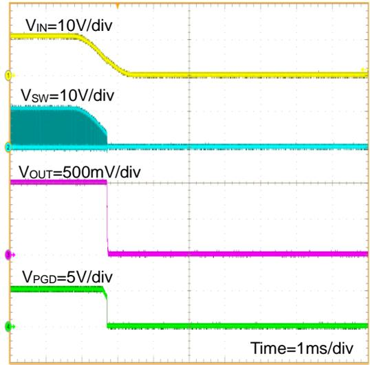
Figure 33. Shutdown Waveform ( $V_{IN}=V_{EN}$ )
