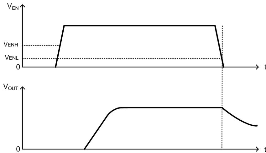
Figure 46. Start Up and Shut Down with Enable
