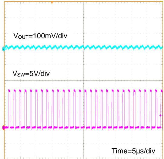
Figure 80.  $V_{OUT}$  Ripple  $I_{OUT}=8A$  ( $V_{IN}=12V, V_{OUT}=3.3V, FREQ=H(600kHz)$ )
