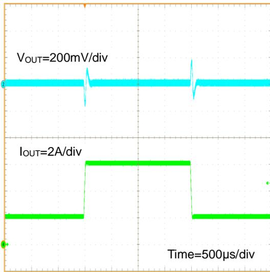
Figure 84. Load Transient Response  $I_{OUT}=2A - 6A$
