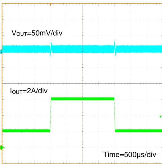
Figure 59. Load Transient Response I<sub>OUT</sub>=2A - 6A (V<sub>IN</sub>=12V, V<sub>OUT</sub>=1V, FREQ=H(600kHz))
