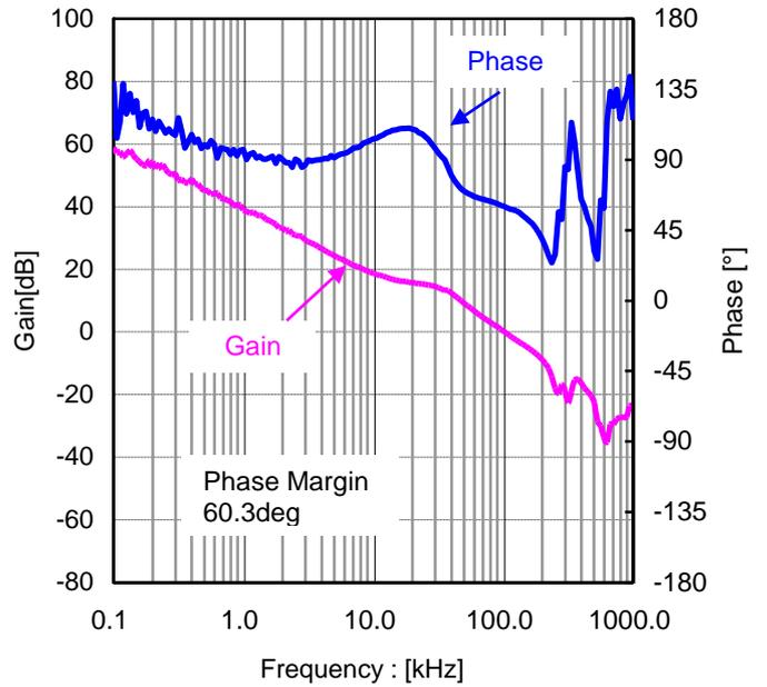
Figure 63. Loop Response  $I_{OUT}=8A$
