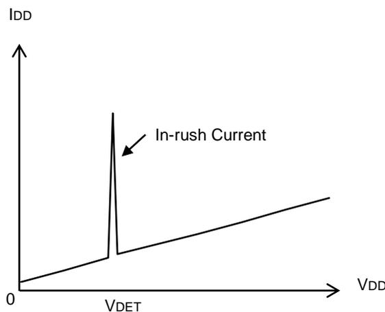
Fig. 22 Current Consumption vs. Power Supply Voltage
