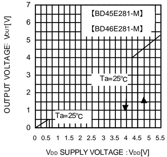
Fig.6 I/O Characteristics
