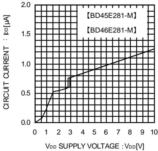
Fig.3 Circuit Current
