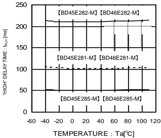
Fig.13 Output Delay Time
