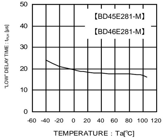
Fig.14 Output Delay Time
