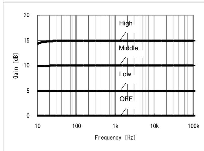
Figure 33. The representative characteristic of Output Gain
