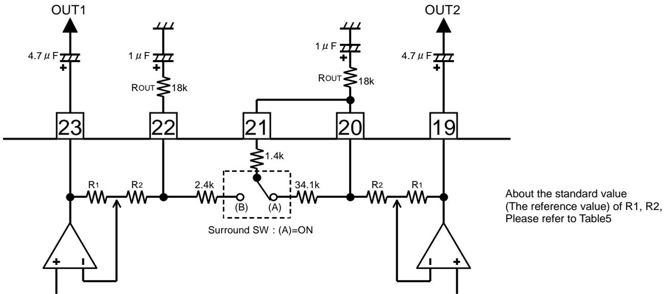
Figure 32. The application circuit example of Output Gain
