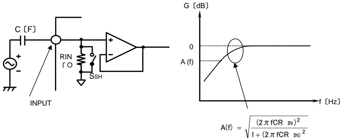
Figure 16. Input short circuit
