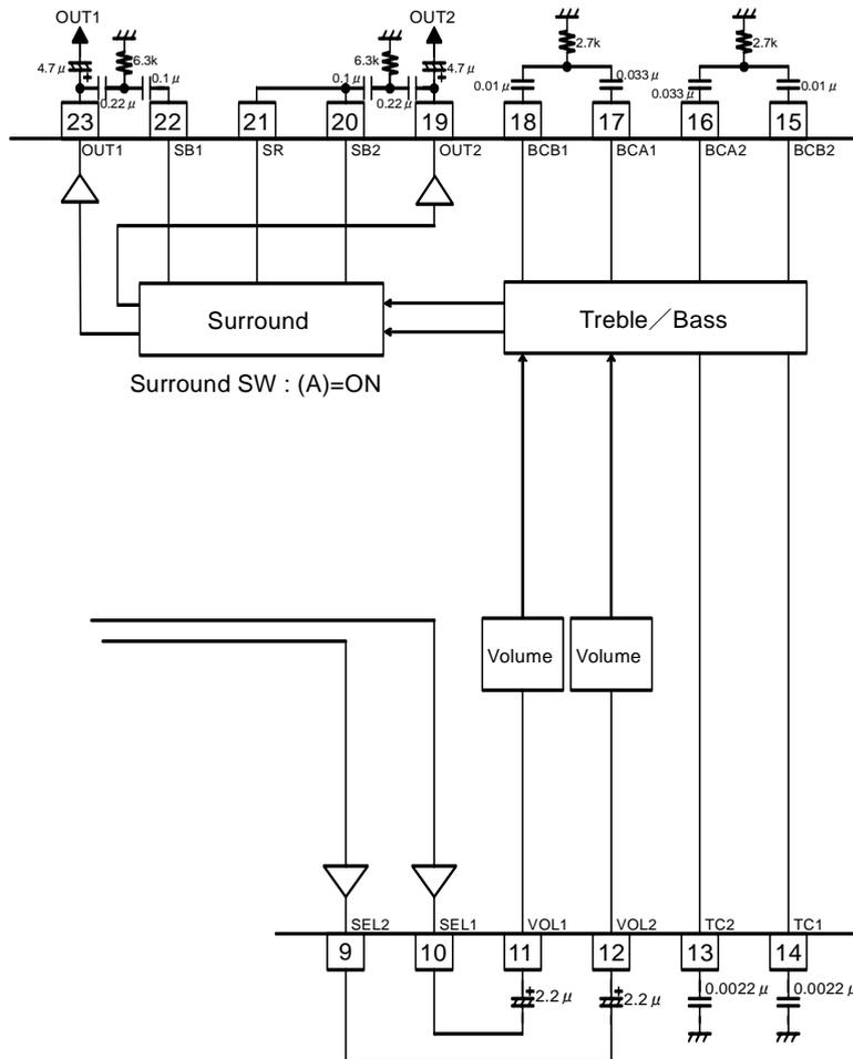
Figure 34. The application circuit example of easy 3band
