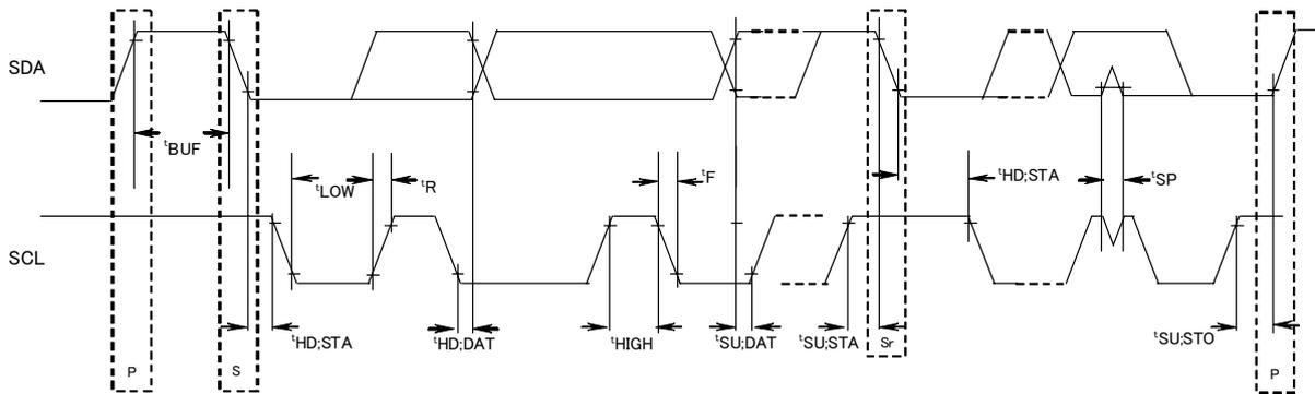
Figure 12. Definition of timing on the I<sup>2</sup>C-bus
