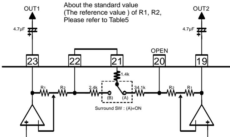
Figure 28. The application circuit example of easy Surround
