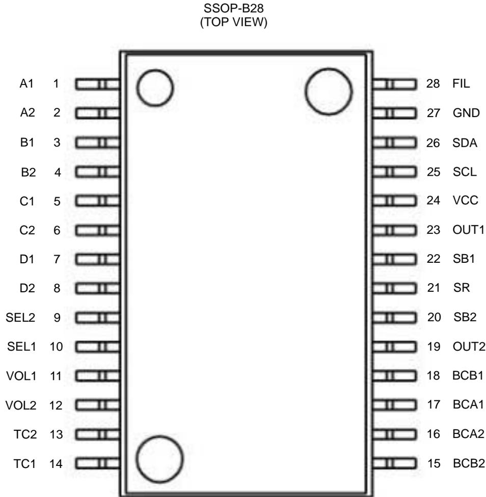
Figure 2. Pin configuration
