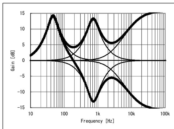
Figure 35. The representative characteristic of easy 3band
