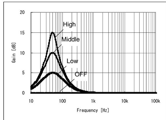
Figure 23. The representative characteristic of Bass Boost
