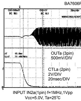
Fig.12 Switching characteristics1
