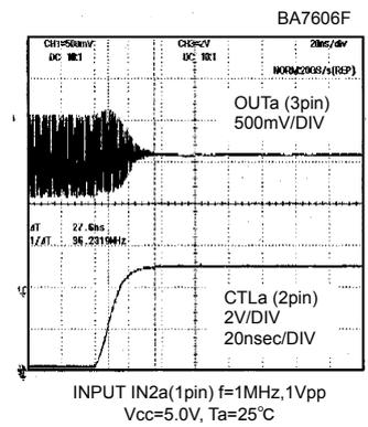
Fig.13 Switching characteristics2
