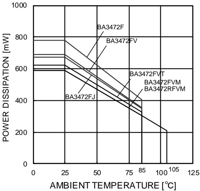
Figure 2. Derating Curve
