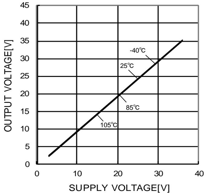
Figure 5. High level Output Voltage - Supply Voltage (RL=10kΩ)
