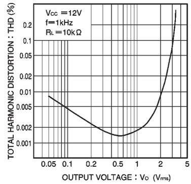
Fig. 14 Total harmonic distortion vs. output voltage
