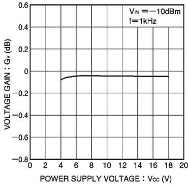
Fig. 10 Voltage gain vs. power supply voltage
