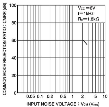
Fig. 17 Common-mode rejection ratio vs. input voltage
