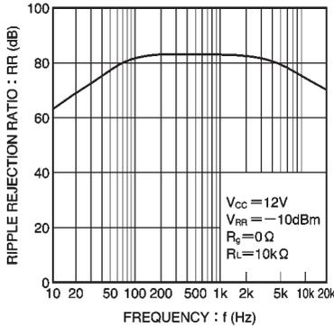
Fig. 13 Ripple rejection ratio vs. frequency
