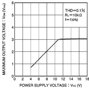
Fig. 8 Maximum output voltage vs. power supply voltage
