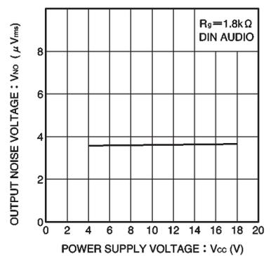
Fig. 9 Output noise voltage vs. power supply voltage
