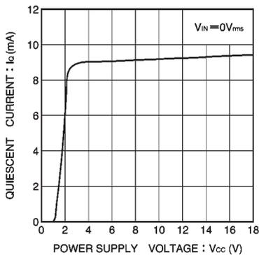
Fig. 7 Quiescent current vs. power supply voltage
