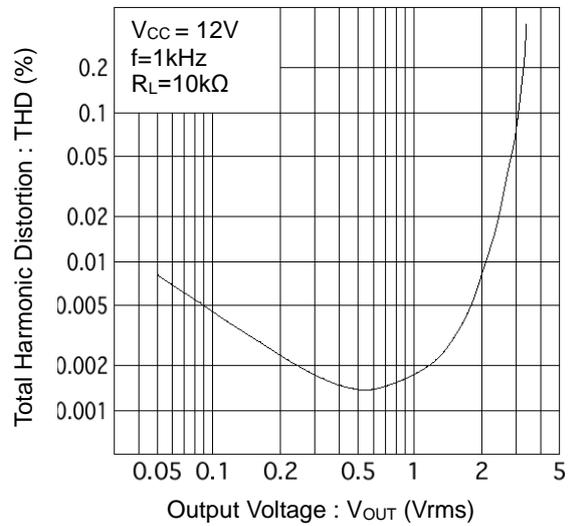
Figure 8. Total Harmonic Distortion vs Output Voltage
