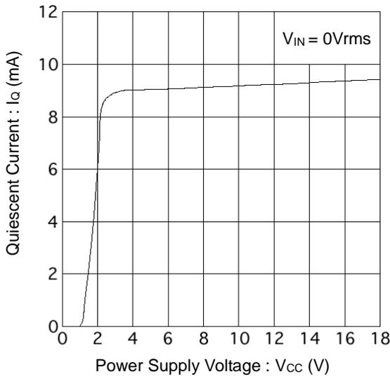
Figure 1. Quiescent Current vs Power Supply Voltage
