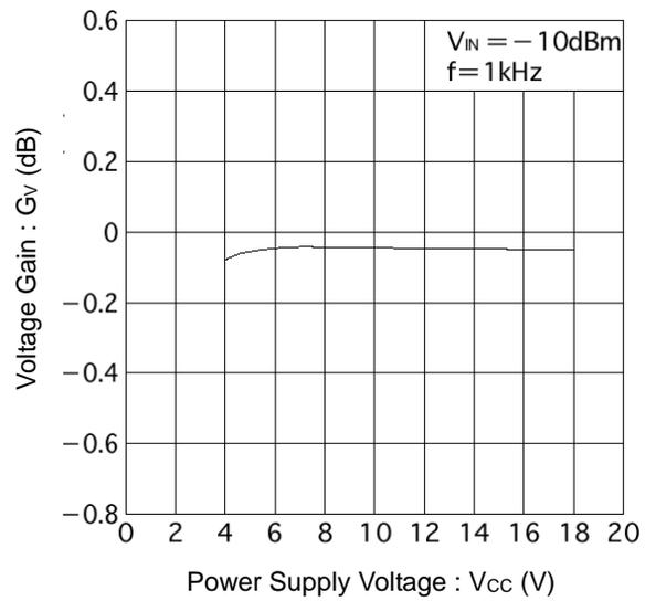
Figure 4. Voltage Gain vs Power Supply Voltage
