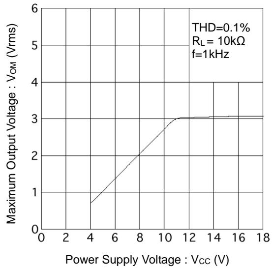
Figure 2. Maximum Output Voltage vs Power Supply Voltage
