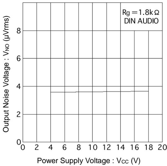
Figure 3. Output Noise Voltage vs Power Supply Voltage
