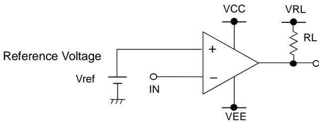
While the input voltage is smaller than the reference voltage, the output voltage remains high. In case the input voltage becomes higher than the reference voltage, the output voltage will turn low.
