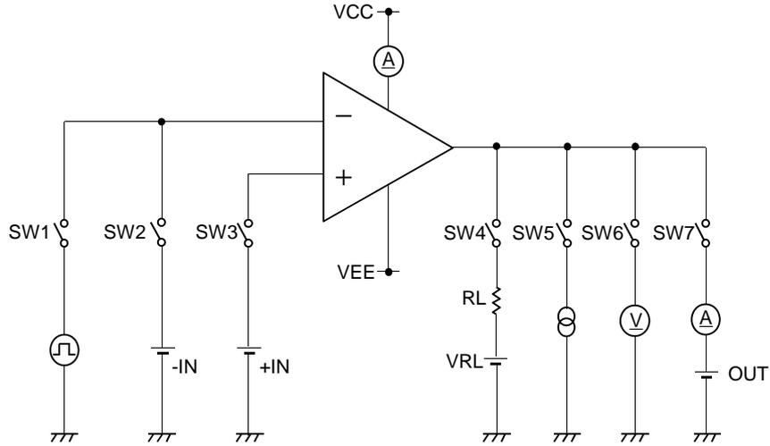
Figure 50. Test Circuit 2 (one channel only)
