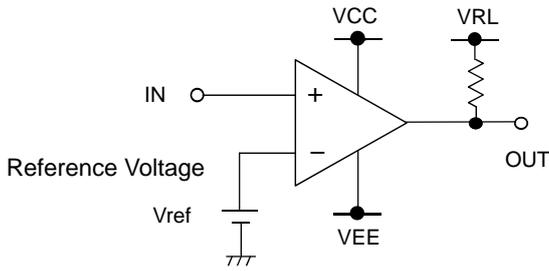
While the input voltage is higher than the reference voltage, the output voltage remains high. In case the input voltage becomes lower than the reference voltage, the output voltage will turn low.
