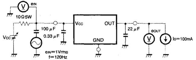
$$\text{Ripple rejection ratio R.R.} = 20 \log \left( \frac{e_{IN}}{e_{OUT}} \right)$$
