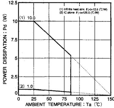
Fig. 7 Ta - power dissipation characteristic (TO 252-3)
