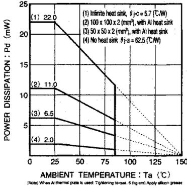
Fig. 6 Ta - power dissipation characteristic (TO220FP)
