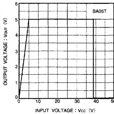
Fig. 10 Over voltage protection characteristic
