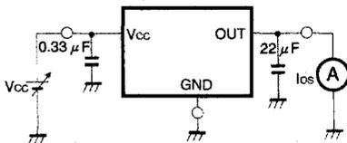
Fig. 5 Measurement circuit for short-circuit output current
