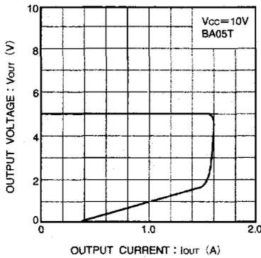
Fig. 9 Current limit characteristic
