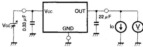
Fig. 1 Measurement circuit for output voltage, line regulation, load regulation, temperature coefficient of output voltage
