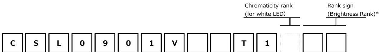
Series name      Package Type      Chip type      Emitting Color      Resin Color Taping Specification
