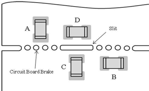
Stress strength according to the mounting position:
