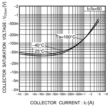
Fig.7 Collector-emitter saturation voltage vs. collector current (III)
