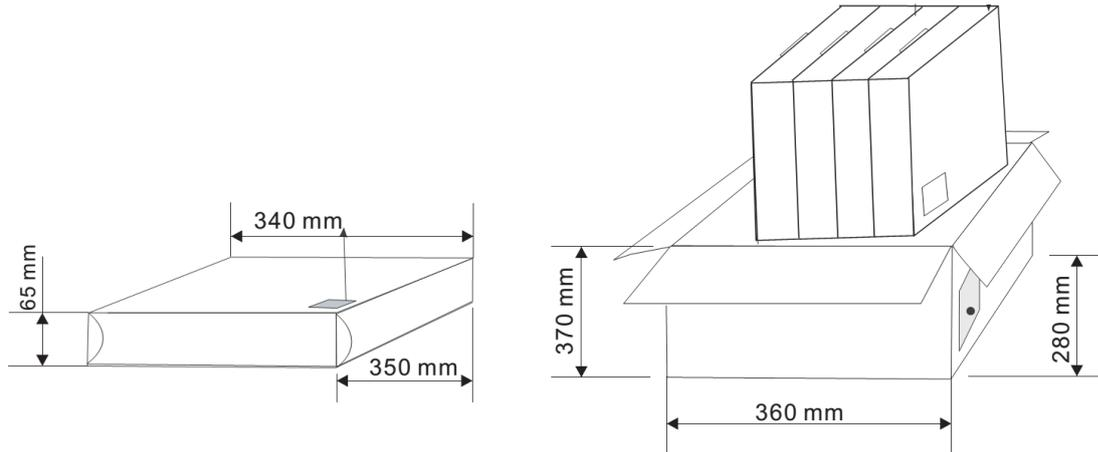
Figure 13: Reel cartons used for type number BMD-330-A-R-00
