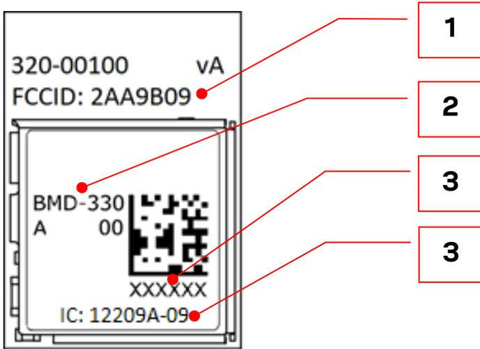
Figure 5: Module marking for type number BMD-330-A-R-00
