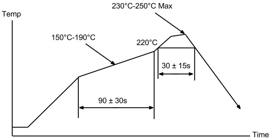
Figure 16: Reflow Profile for Lead Free Solder
