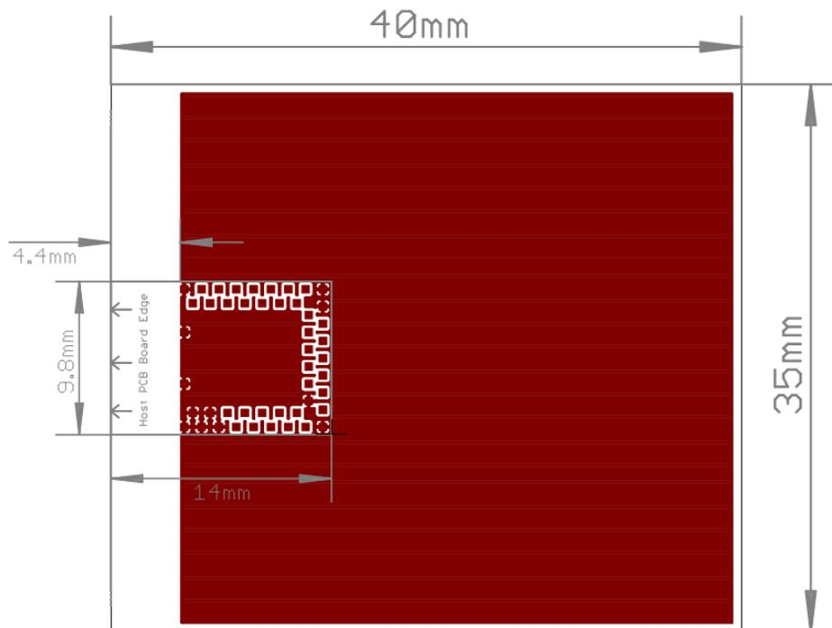
Figure 8: Recommended RF layout and ground plane
