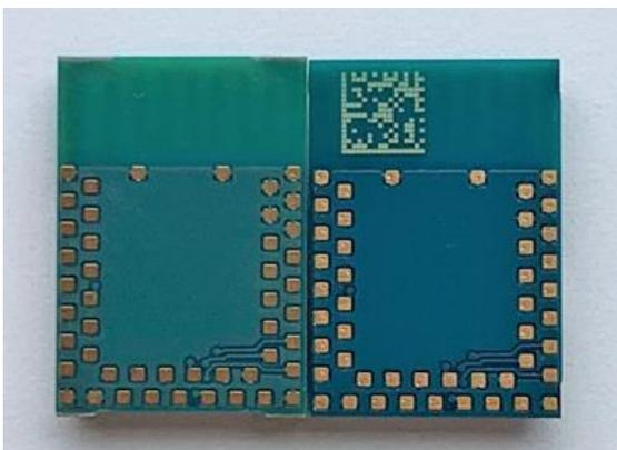
Figure 7: Bottom data matrix on type number BMD-330-A-R-20
